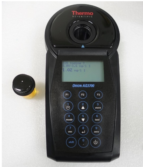
Figure 4.28: Thermo Scientific colorimetry meter used for sulfate testing
