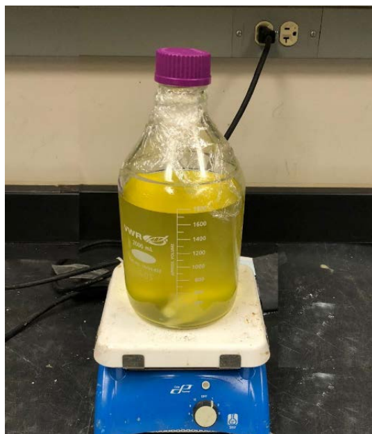
Figure 3.3: AAS being magnetically stirred at room temperature
