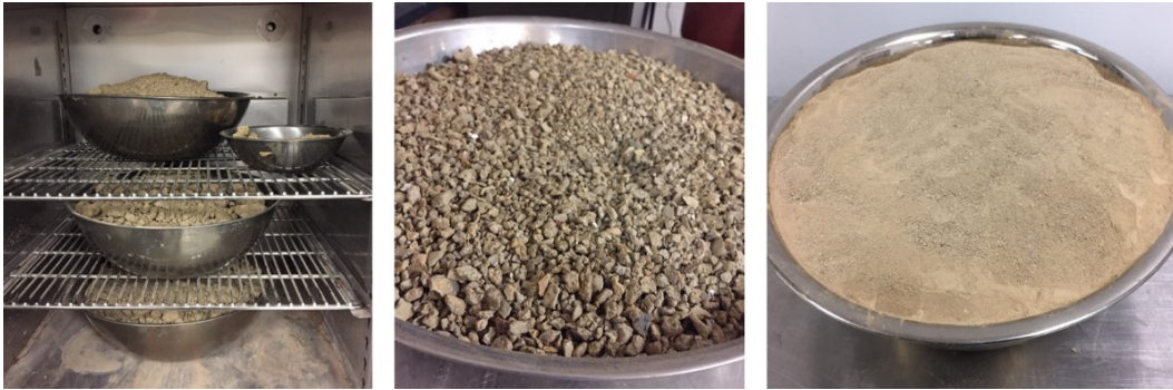
Figure 4.3: Soils oven-dried, crushed, and pulverized before testing.
