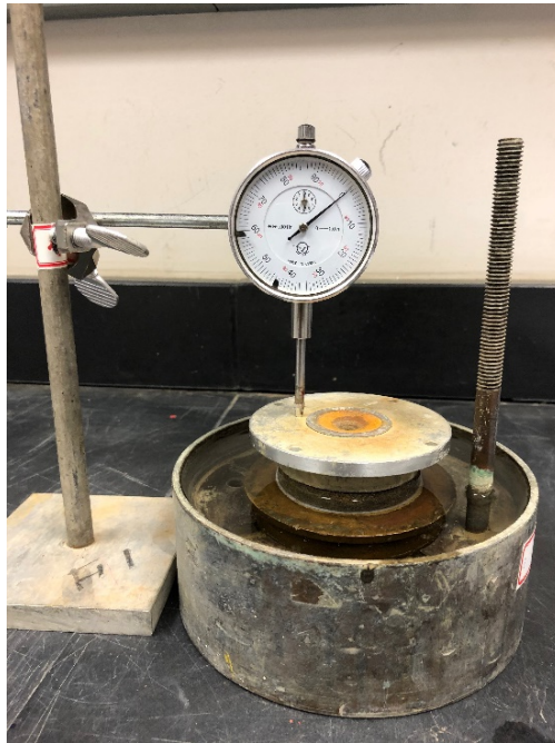
Figure 4.21: Modified 1-D swell test setup
