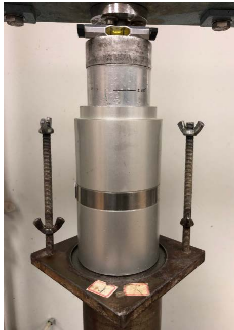
Figure 4.18: Static compaction of specimens for engineering tests
