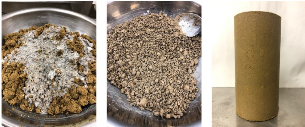
Figure 4.27: Process of mixing geopolymer slurry with soil to make test specimen
