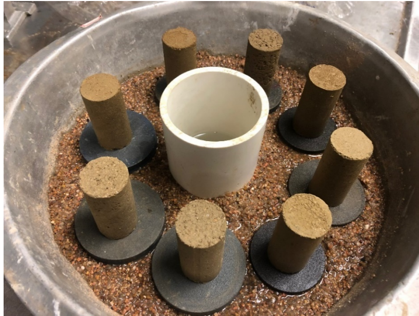
Figure 4.23: Modified durability test setup using capillary soaking
