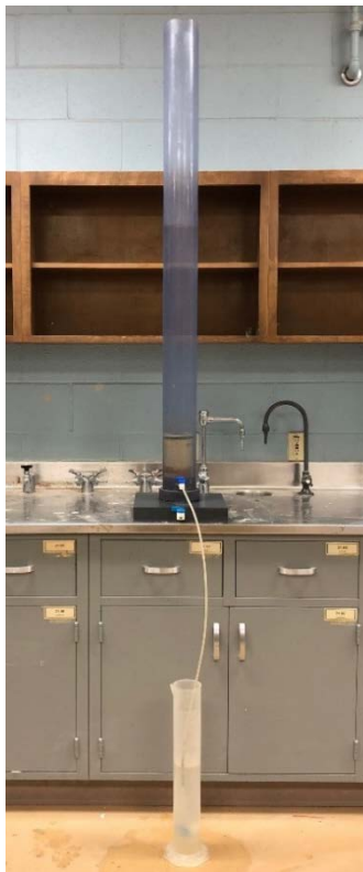
Figure 4.26: Modified leachability test setup
