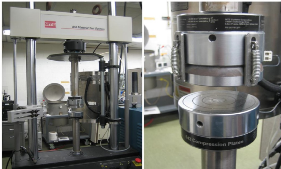
Figure 3.7: 810 MTS system used for strength testing of geopolymer specimens
