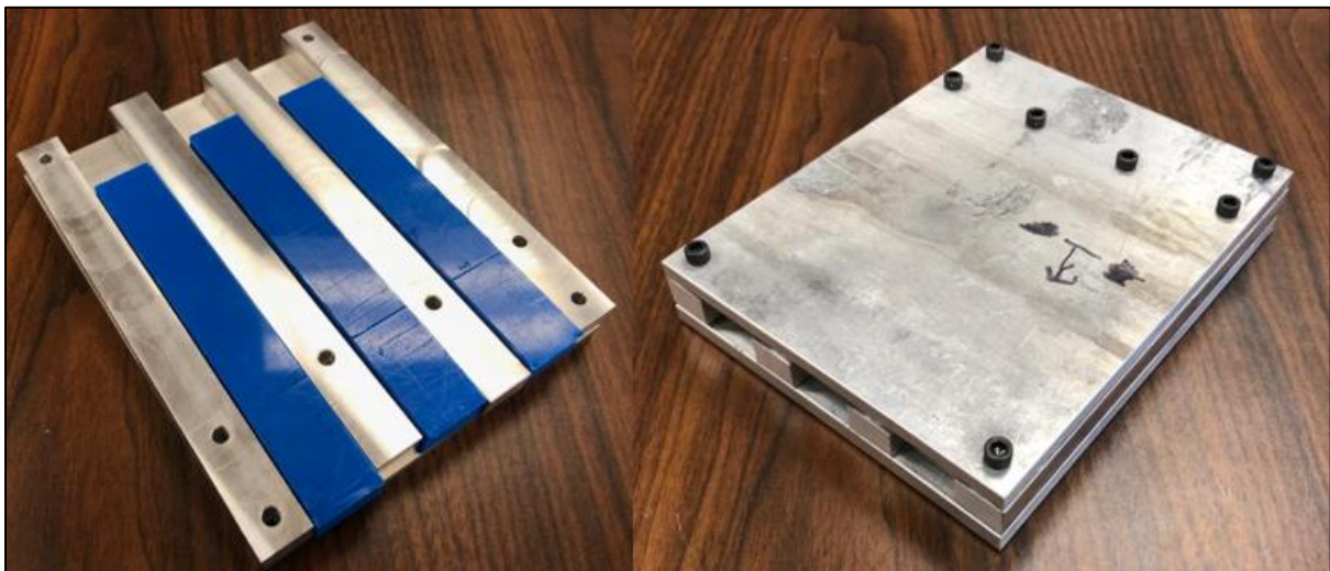
Figure 25: Heat treatment fixture
