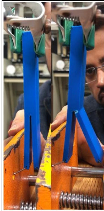
Figure 15: Failure of initial DCB specimen design
