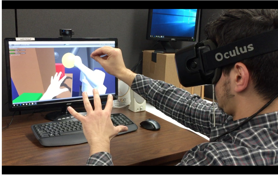
Figure 1.4. A human operator teaches a robot in VR simulation. Figure reproduced from [8].
