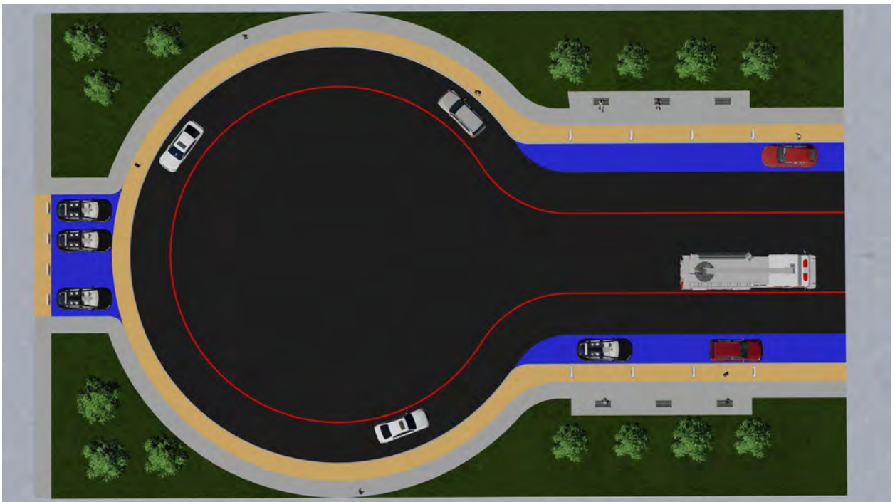
Figure 39 Fire Lane Recommendation Plan View
