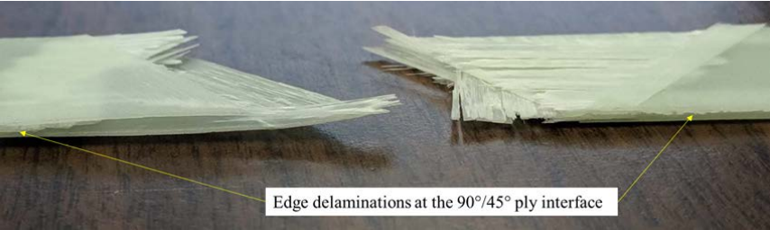
Figure 4.9 Edge delaminations at the 90°/45° ply interface that grows along the width to induce fracture
