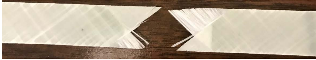
Figure 4.13 Fractured off axis laminate
