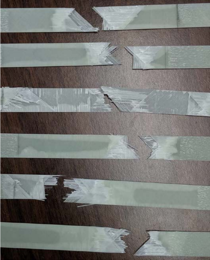
Figure 4.10 Fractured quasi isotropic laminates
