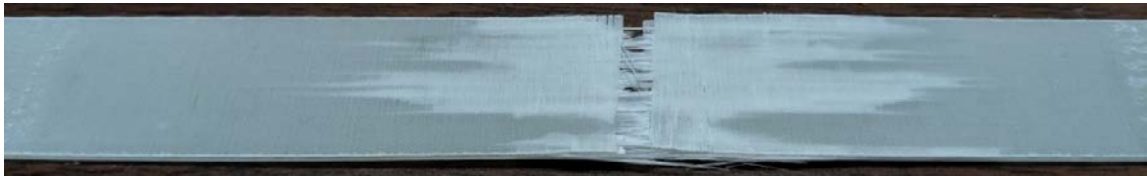
Figure 4.5 Fractured cross ply laminate showing transverse cracks, delaminations and fiber splits
