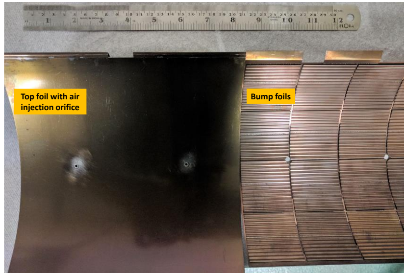
Figure 58 Top foil and bump foil assembly showing injection orifice
