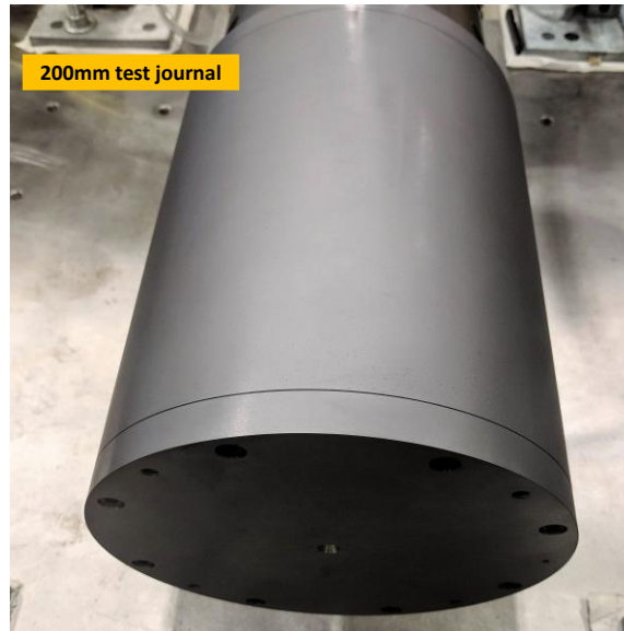
Figure 63 200 mm OD test journal
