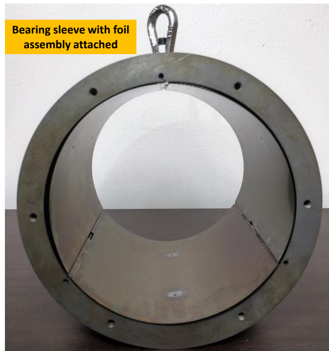
Figure 59 Bearing sleeve with foils attached
