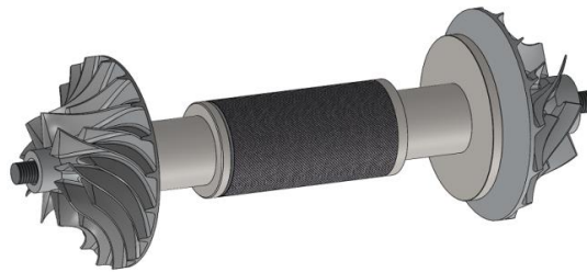
Figure 43 Scale model of 1.5 MW medium pressure compressor with foil bearings
