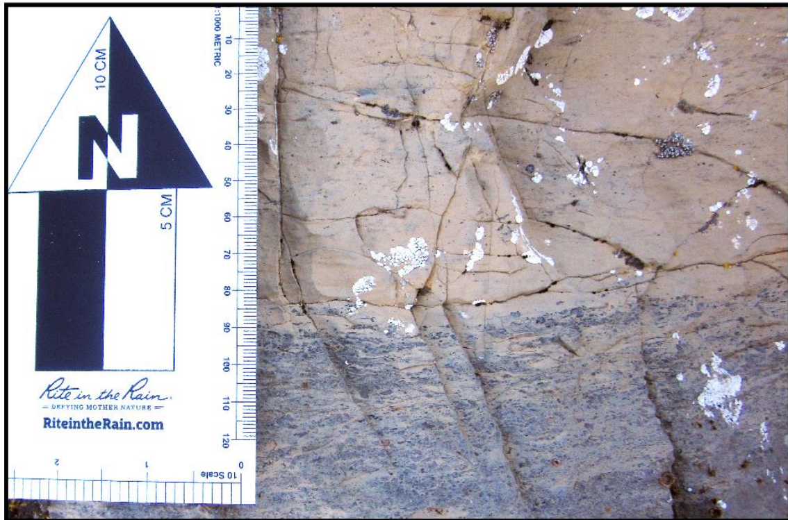
Figure 3.9 – Gradational transition from gray, fossiliferous, nearly nodular wackestone to a thin layer of tan, interbedded calcareous siltstone (unit 1; upper part of the Ely Limestone) (right side of scale bar in mm).
