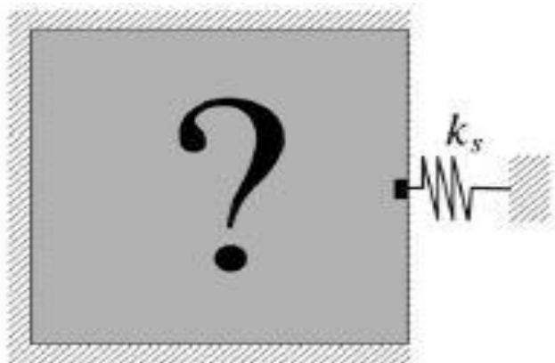
Figure 2-9(a) Thermal actuator design domain [1]
