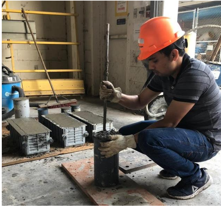
Figure 9 Casting of Cylinder Specimen
