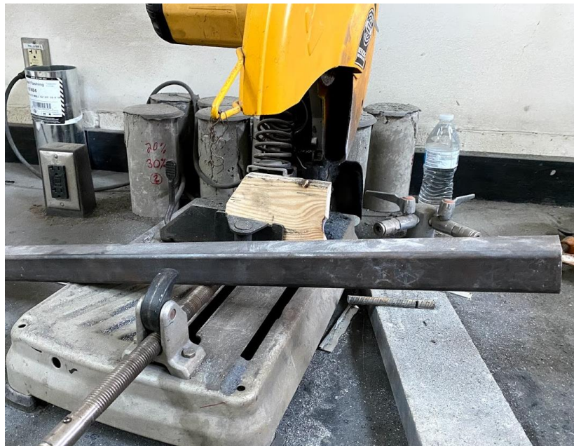
Figure 21 HSS Steel Section
