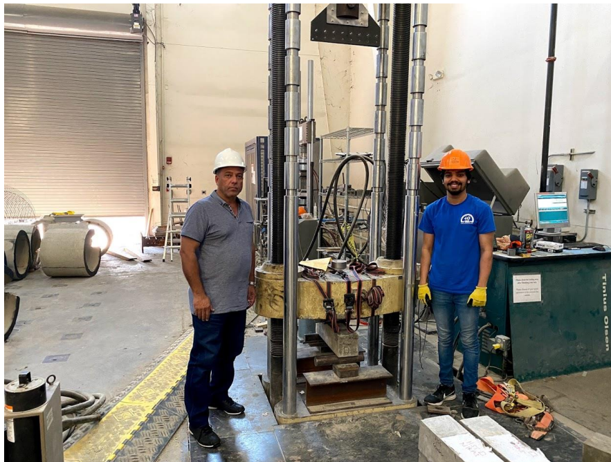
Figure 30 Flexural Test Setup for Concrete Beams
