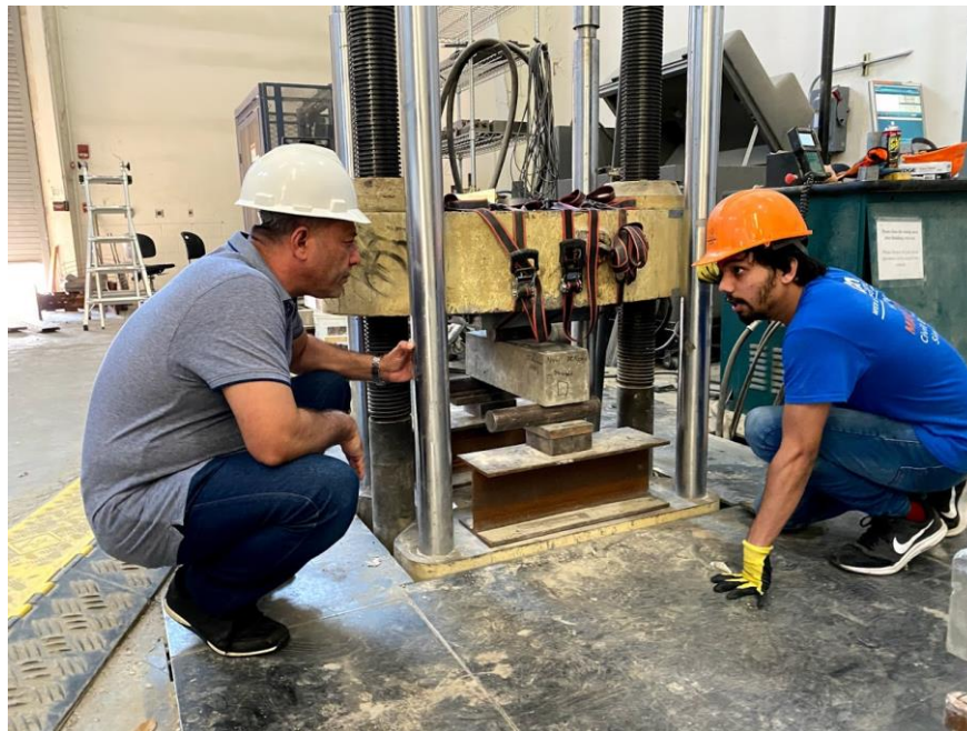
Figure 28 Flexural Test Setup for Concrete Beams
