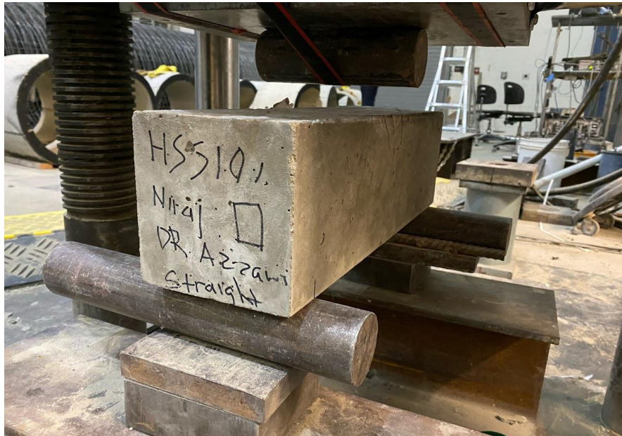
Figure 27 Beams failure and crack formation of 1.0% straight beam at peak load
