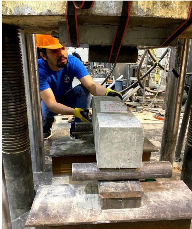
Figure 23 Test setup for Flexure test
