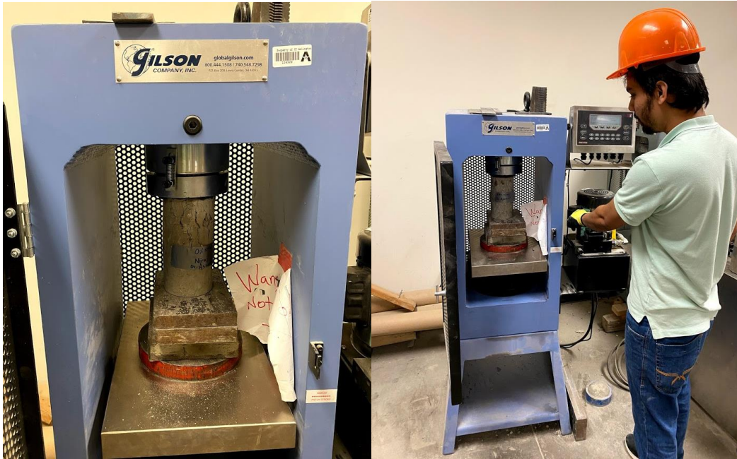
Figure 13 Cylinder Compression (4" x 8") Test Setup
