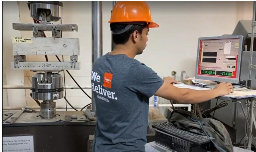
Figure 17 Modulus of Rupture Test Setup
