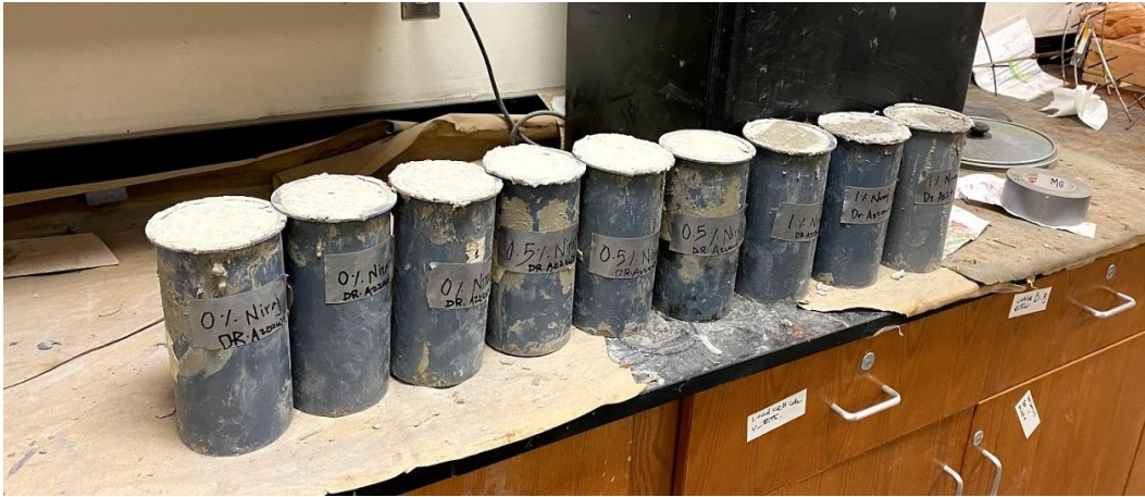
Figure 11 Cylinders after 28 days
