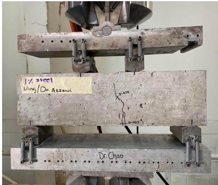
Figure 19 Specimen at Ultimate Load
