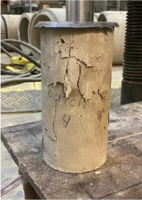
Figure 4.3 Sample Failure After Testing Machine Readjustment
