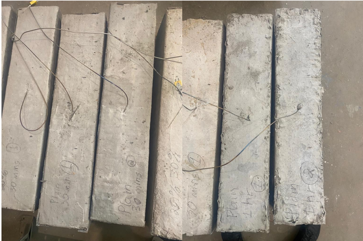
Figure 4.17 Samples with Regular Concrete Exposed to Heat for 30 Minutes (Left) and Samples Exposed to Heat for 1 Hour (Right)
