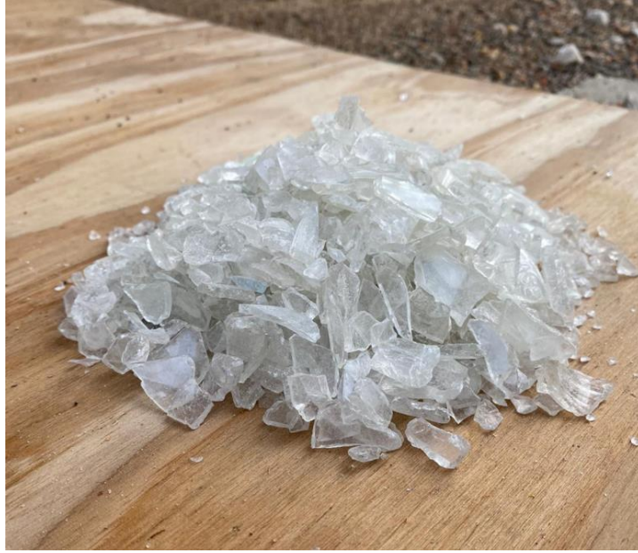
Figure 3.2 Glass Aggregate Used as Coarse Aggregate Replacement
