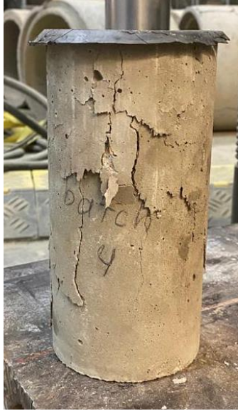
Figure 4.6 Concrete with 20% Glass Powder Replacement Type 2 Fracture Type
