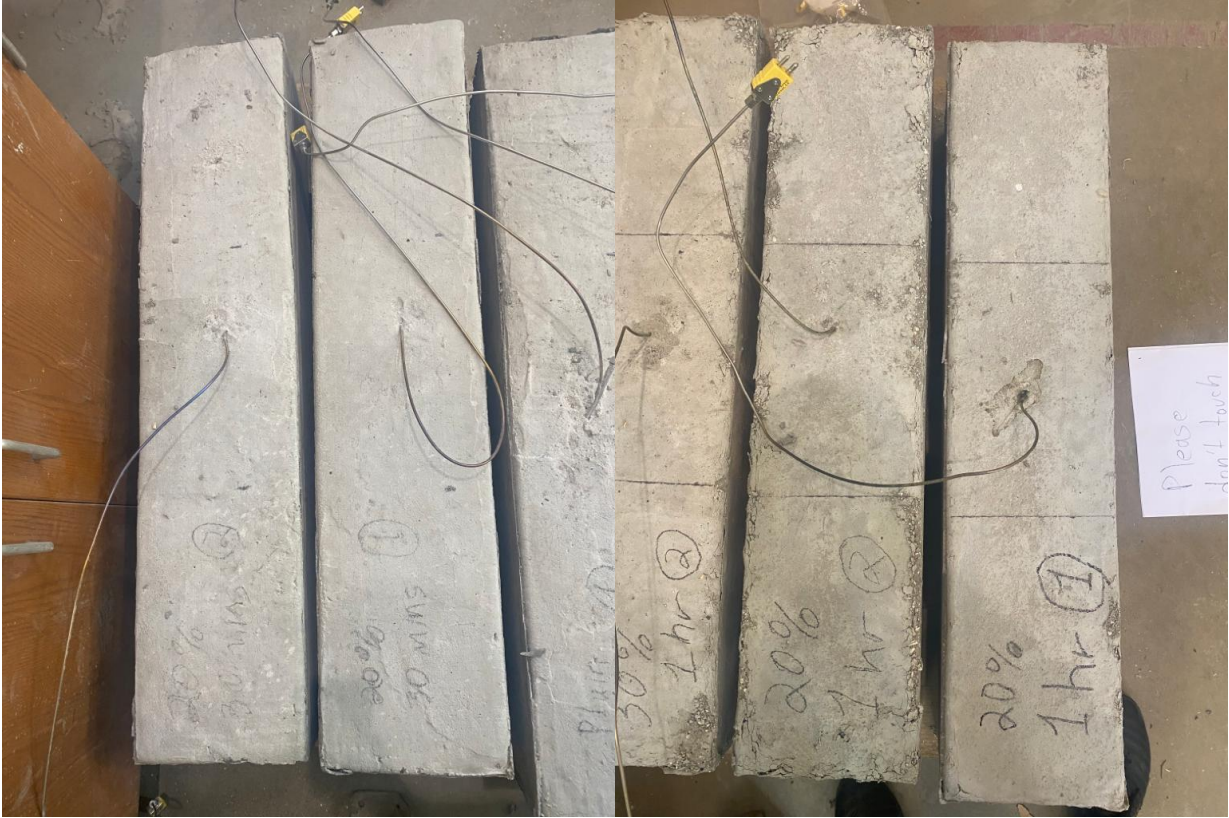
Figure 4.15 Samples with 20% Glass Pozzolan Exposed to Heat for 30 Minutes (Left) and Samples Exposed to Heat for 1 Hour (Right)
