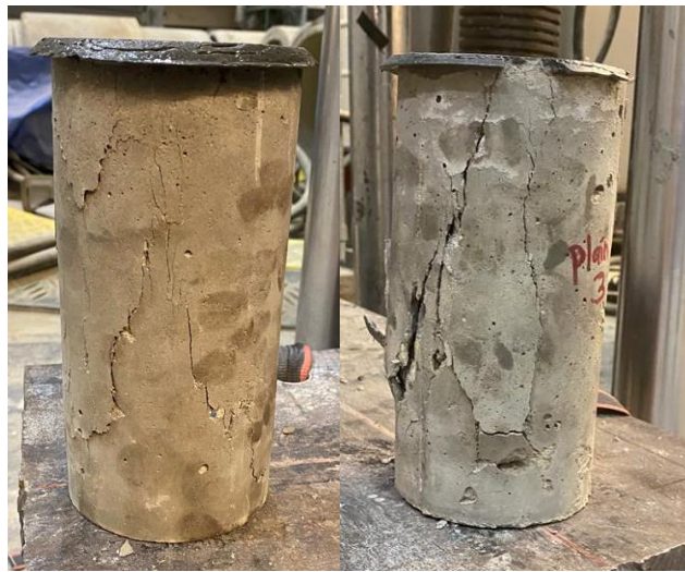
Figure 4.5 Plain Concrete Fracture Patterns Type 2 (Left) and Type 3 (Right)
