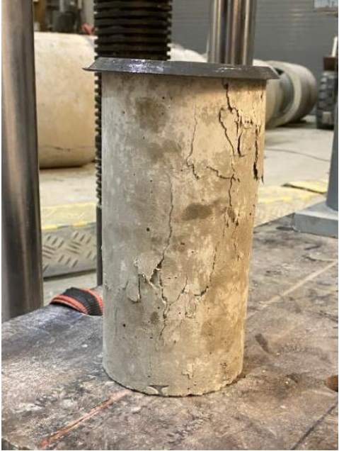
Figure 4.2 Sample Failure Before Testing Machine Readjustment
