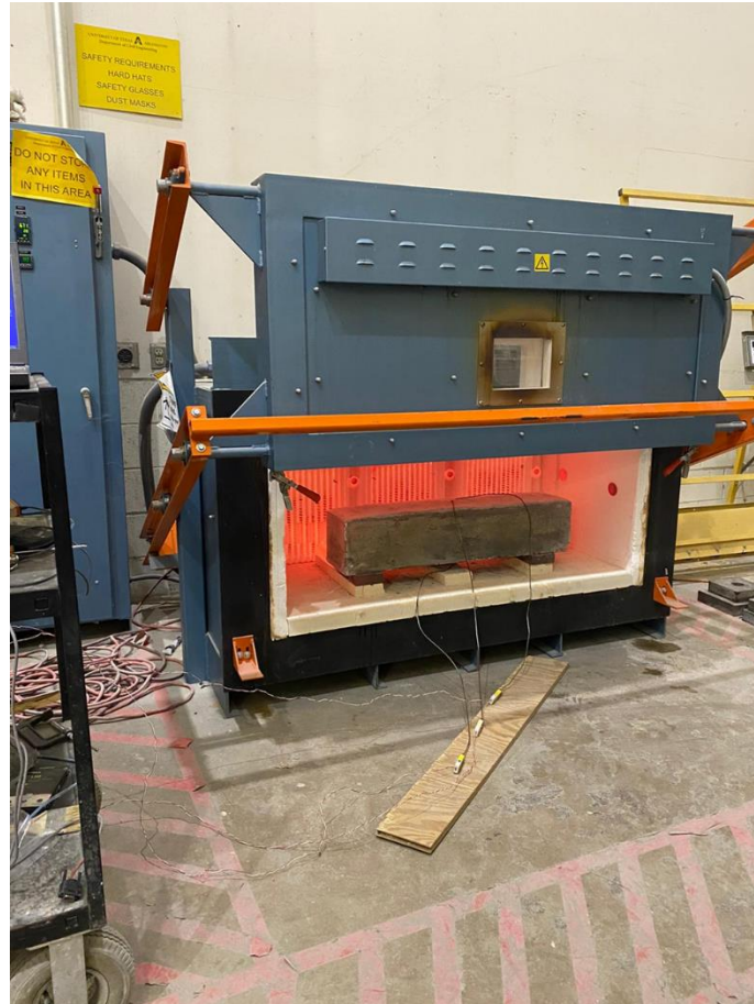
Figure 3.19 Beam Immediately After Heat Treatment
