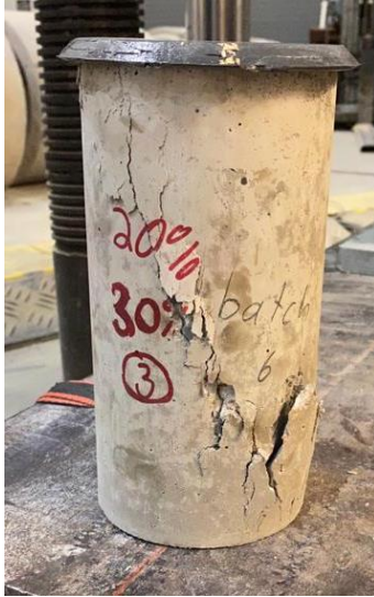
Figure 4.7 Concrete with 20% Glass Powder and 30% Glass Aggregate Failure
