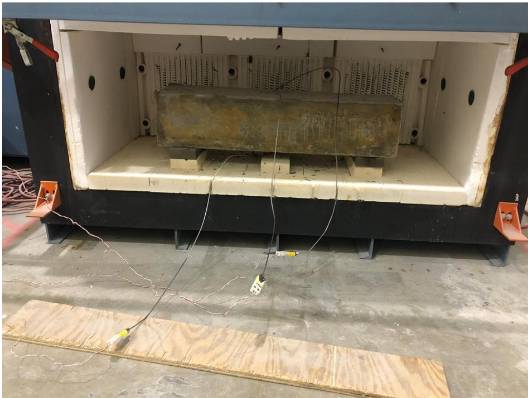
Figure 3.18 Beam Set Up for Heat Treatment
