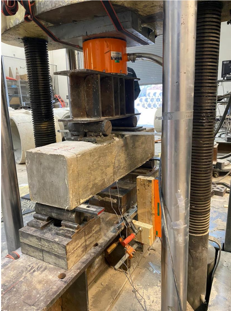
Figure 3.23 Flexural Test Set-Up with Beam
