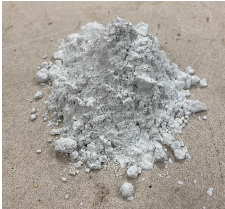
Figure 3.3 VCAS Glass Pozzolan Used as Cement Replacement
