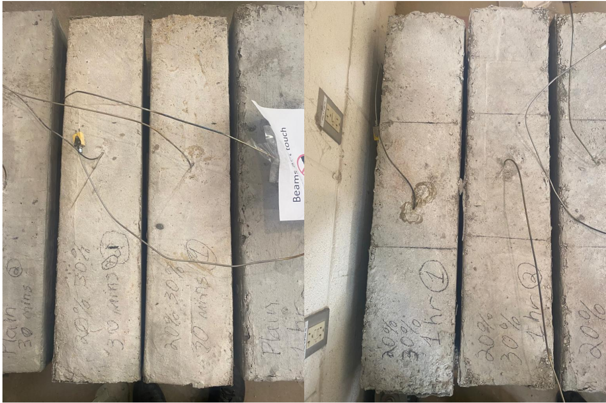
Figure 4.16 Samples with 20% Glass Pozzolan and 30% Glass Aggregate Exposed to Heat for 30 Minutes (Left) and Samples Exposed to Heat for 1 Hour (Right)
