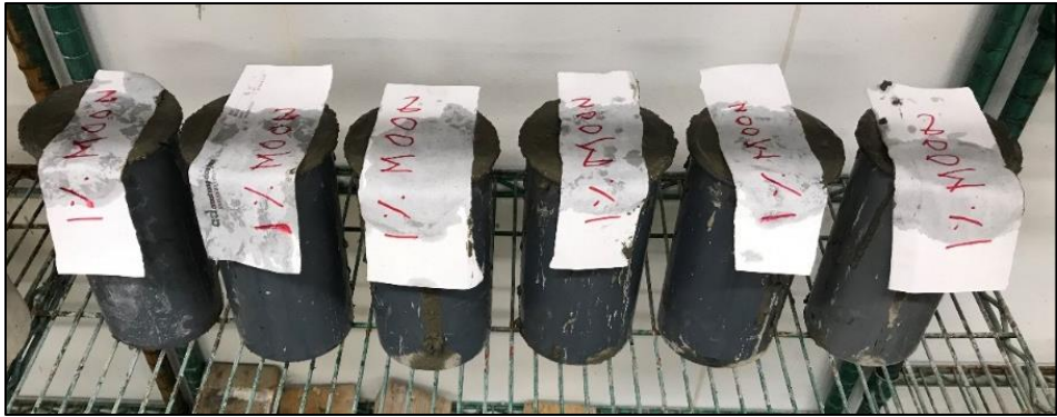
Figure 13. 1.0% SFRC - Cylinder Molds (4" x 8") for Compressive Strength and Split Test
