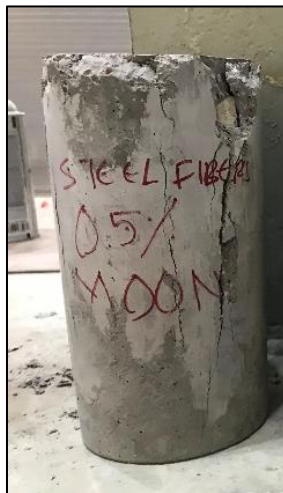
Figure 26. 0.5% SFRC - Cylinder (4" x 8") after testing
