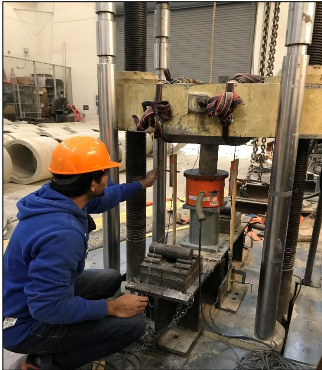
Figure 25. 0.5% SFRC - Cylinder (4" x 8") with Strain gauge and LVDT for Compression Strength Test Setup
