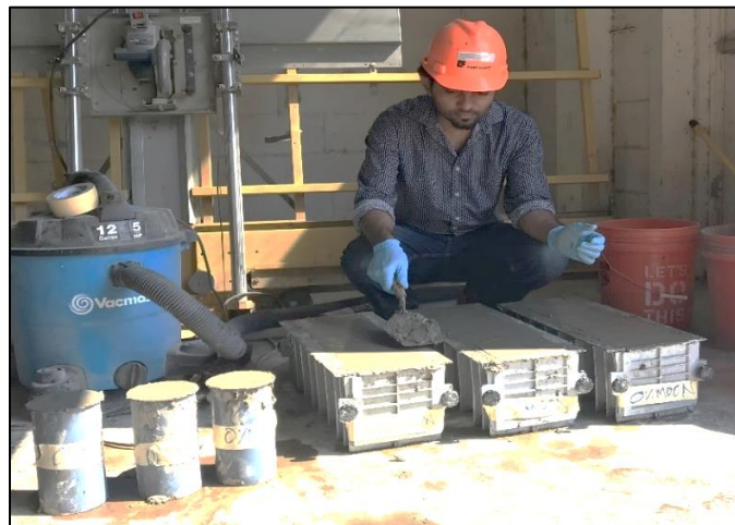
Figure 8. 0.0% SFRC - Beam (6"x6"x21") for Flexure and Cylinder Molds (4" x 8") for Split Test
