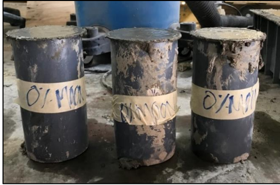
Figure 9. 0.0% SFRC - Cylinder Molds (4" x 8") for Split Test
