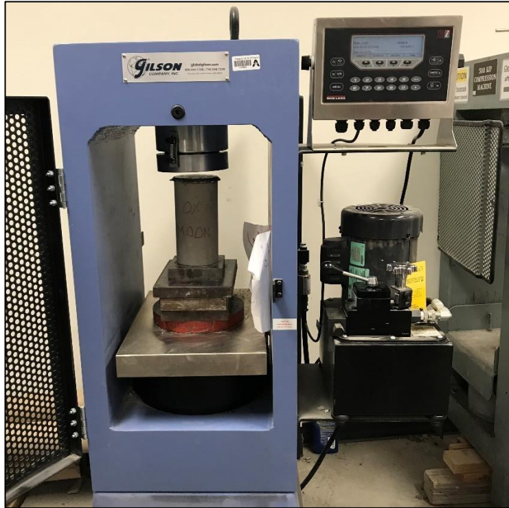
Figure 17. Compression Testing Machine with 0.0% SFRC - Cylinder (4" x 8")
