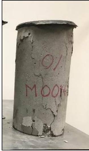
Figure 18. 0.0% SFRC - Cylinder (4" x 8") Collapses after testing
