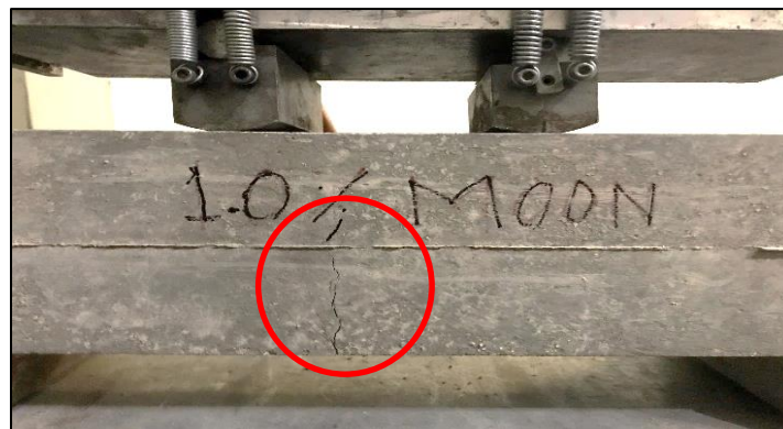
Figure 38. 1.0% SFRC Beam at Failure Load 9.01 Kips
