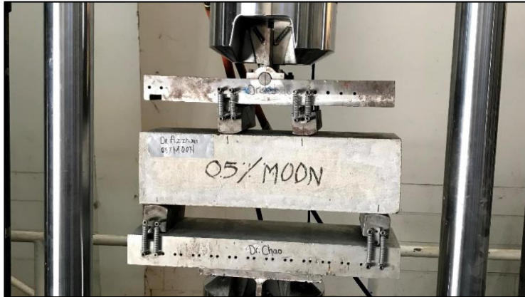
Figure 35. 0.5% SFRC Beam-Modulus of Rupture Test Setup
