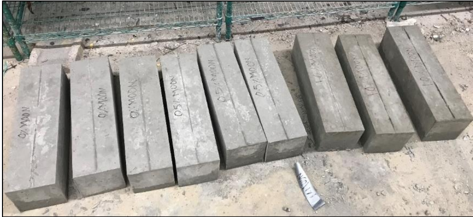
Figure 14. 0.0 %, 0.5% and 1.0% SFRC - Beam Molds (6"x6"x21") for Flexure Test
