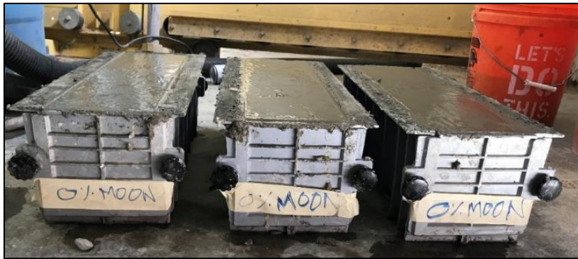
Figure 10. 0.0% SFRC - Beam Molds (6"x6"x21") for Flexure Test
