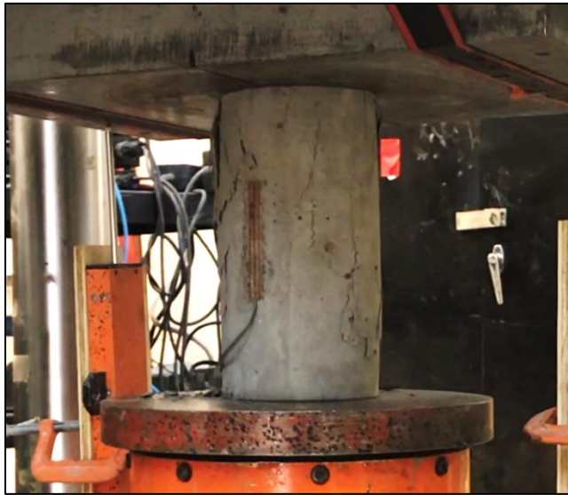
Figure 28. 1.0 % SFRC Cylinder (4" x 8") collapses at 54.29 kips
