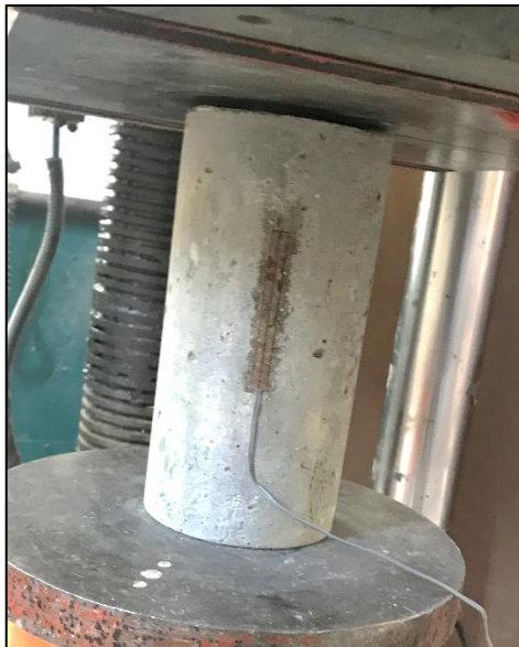
Figure 22. Strain Gauge assembled on Cylinder specimen.
