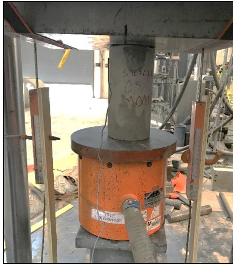
Figure 24. 0.5% SFRC Cylinder (4" x 8") with Strain gauge and LVDT Test Setup
