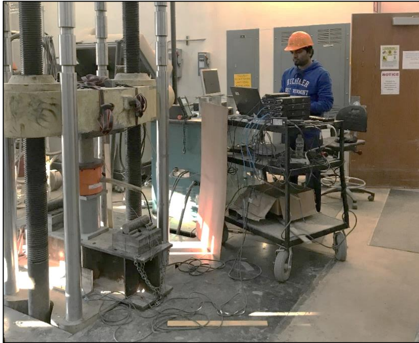
Figure 29. 1.0 % SFRC - Cylinder (4" x 8") with Strain gauge and LVDT for Compression Strength Test Setup
