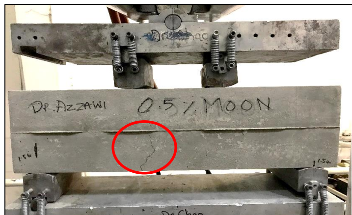
Figure 36. 0.5% SFRC Beam at Failure Load 7.57 Kips
