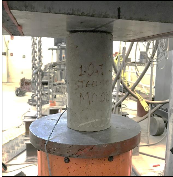
Figure 27. 1.0 % SFRC Cylinder (4" x 8") with Strain gauge and LVDT Test Setup
