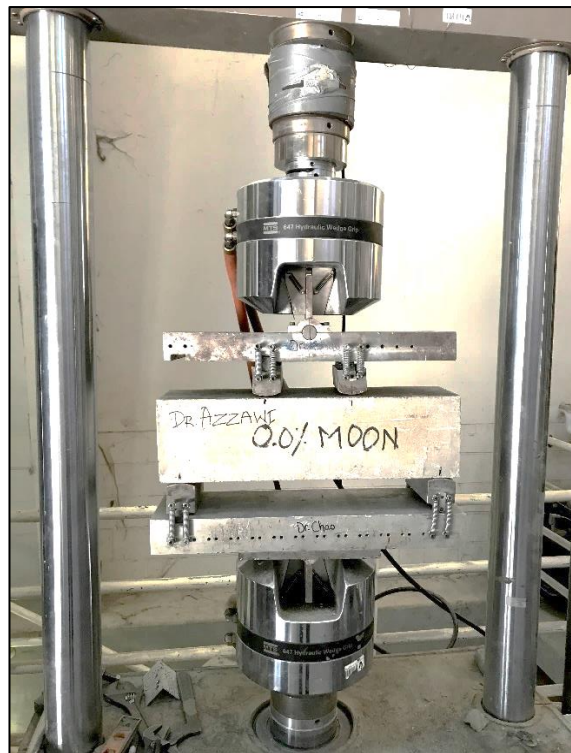
Figure 33. 0.0% SFRC Beam-Modulus of Rupture Test Setup
