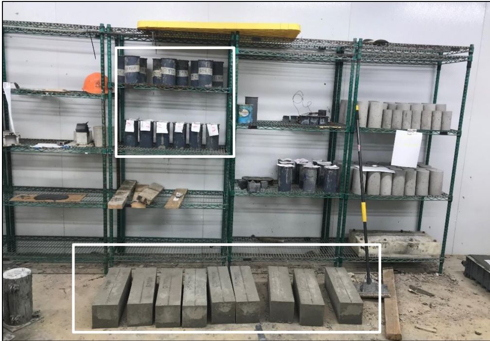
Figure 16. Humidity-Controlled Room (Specimens marked in white boxes)
