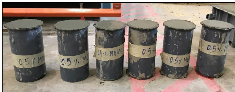
Figure 11. 0.5% SFRC - Cylinder Molds (4" x 8") for Compressive Strength and Split Test
