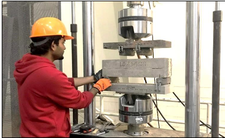
Figure 37. 1.0% SFRC Beam-Modulus of Rupture Test Setup
