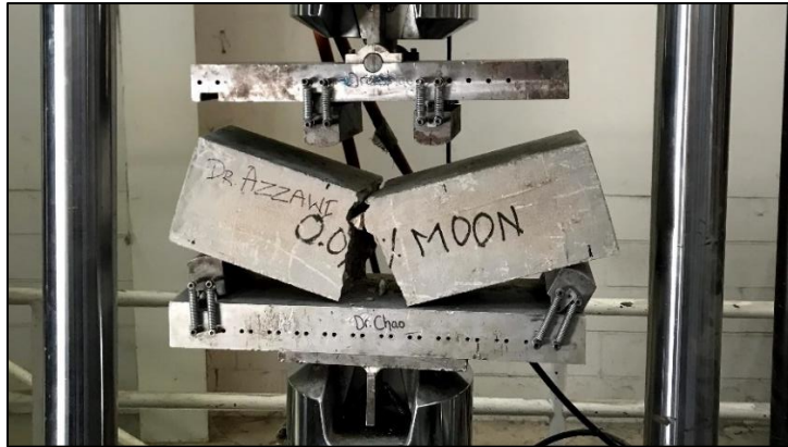
Figure 34. 0.0% SFRC Beam at Failure Load 6.82 Kips
