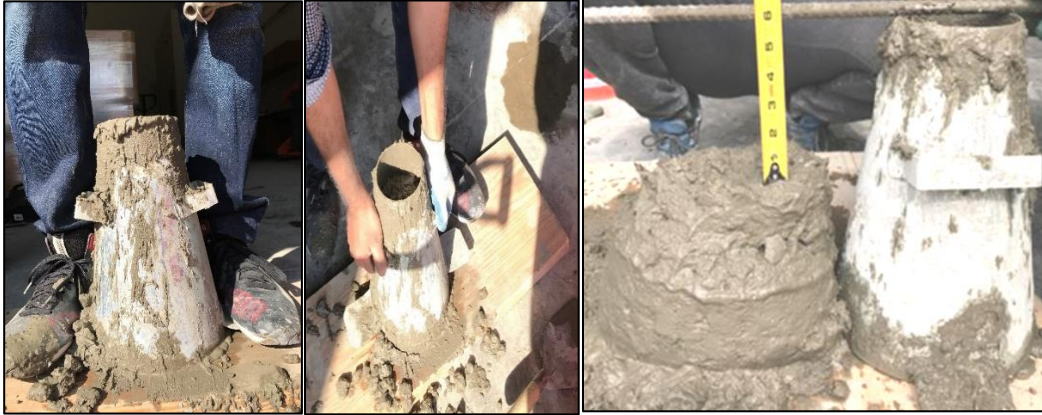
Figure 15. Slump Test on 0.5 % Steel Fiber Concrete Mix
