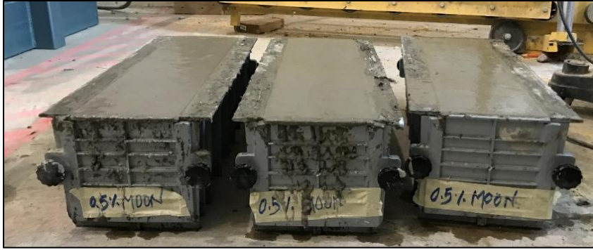
Figure 12. 0.5% SFRC - Beam Molds (6"x6"x21") for Flexure Test
