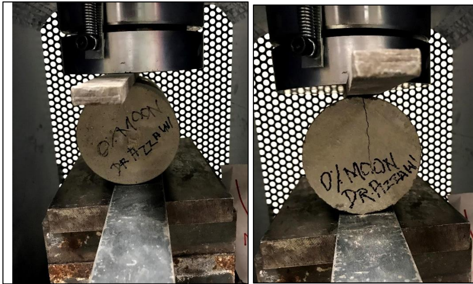
Figure 30. Split Tensile Setup- 0.0 % SFRC - Cylinder (4" x 8")
