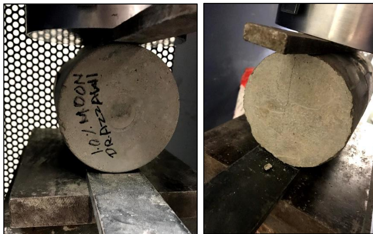
Figure 32. Split Tensile Setup- 1.0 % SFRC - Cylinder (4" x 8")
