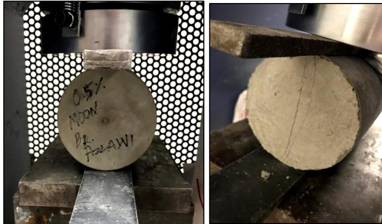
Figure 31. Split Tensile Setup- 0.5 % SFRC - Cylinder (4" x 8")
