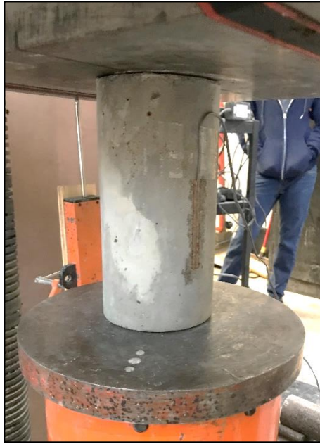
Figure 23. 0.5% SFRC – Cylinder (4" x 8") with a Strain gauge.
