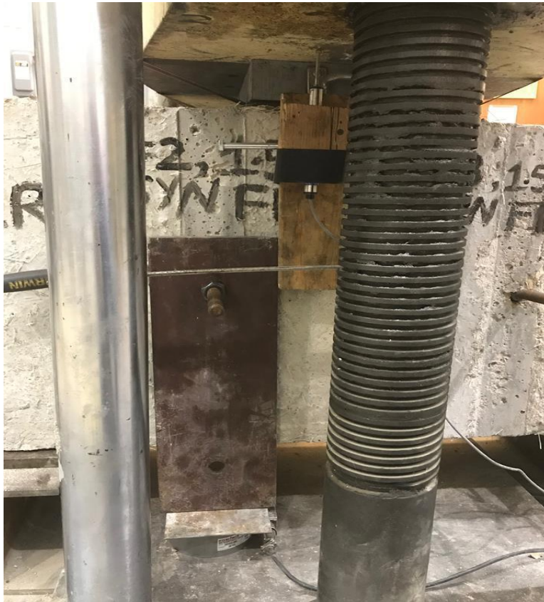
Figure 10. Load cell placement (Khanfar M. et al. 2019)
