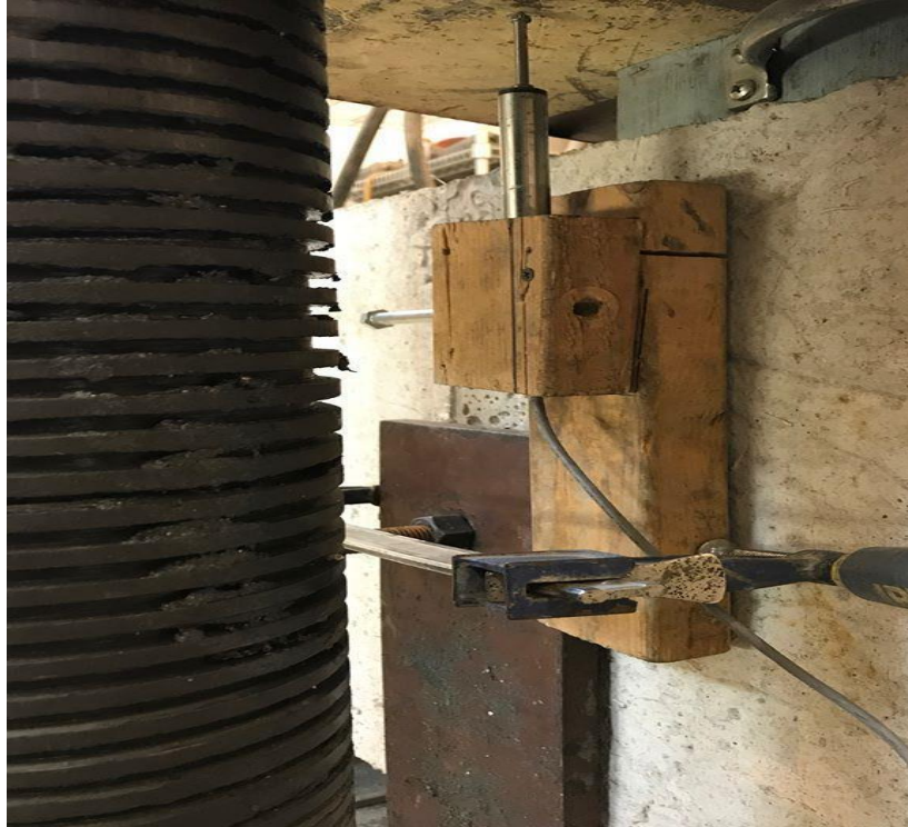
Figure 11. Linear Variable Differential Transformers (LVDT) placement (Khanfar M. et al. 2019)
