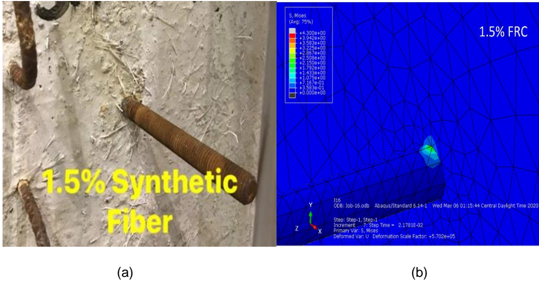
Figure 45. (a) Experiment test of 1.5% SYN-FRC Beam (Khanfar M. et al. 2019) (b) Abaqus Model for 1.5% SYN-FRC Beam
