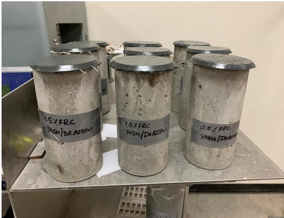
Figure 8. Capping of Specimens for Compression test
