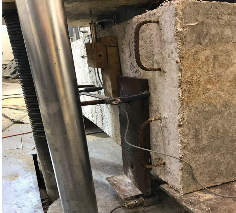
Figure 12. Linear Variable Differential Transformers (LVDT) and Load Cell Setup (Khanfar M. et al. 2019)
