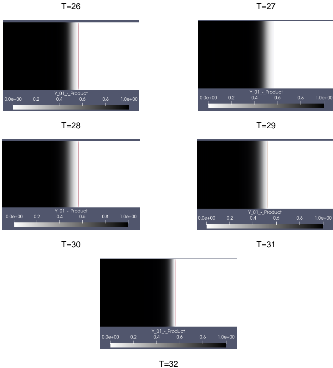
Figure 3-16 Sequence of Reinitiation of Detonation E_a = 26 using Pressure Gradient and Product Contour
