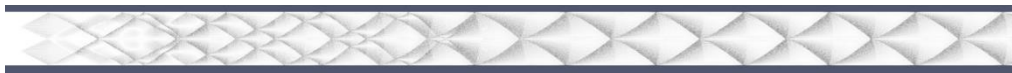
Figure 4-13 Numerical Soot Foil Showing of H_2 - O_2 - 7Ar @6.67 kPa using Inviscid, Global One Step Model
