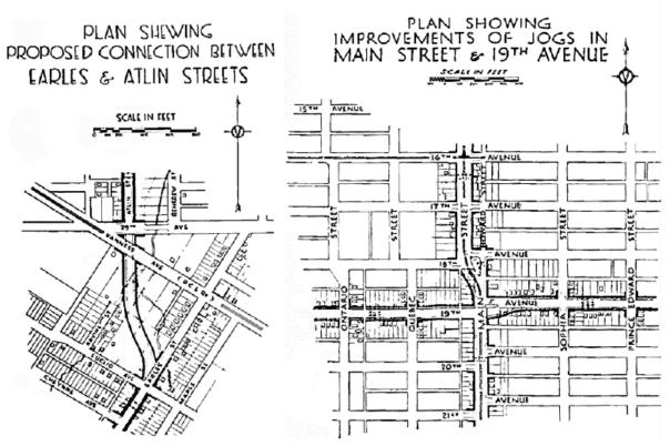
Figure 3.3: Two examples of revised street configurations proposals intended to improve traffic flow on city streets in Vancouver at specific intersections (Bartholomew, 1929).
