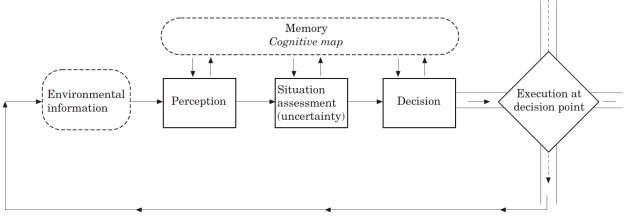
FIGURE 1. Model of wayfinding while driving.
