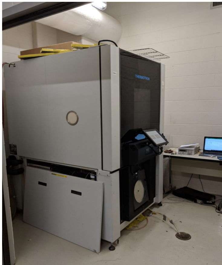
Fig 8-2: Thermotron SE-600-10-10 Environmental Chamber
