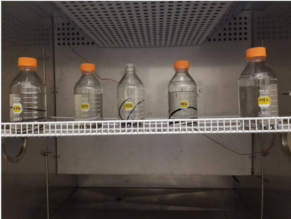
Fig 10-1: Thermal cycling setup inside the Thermotron chamber
