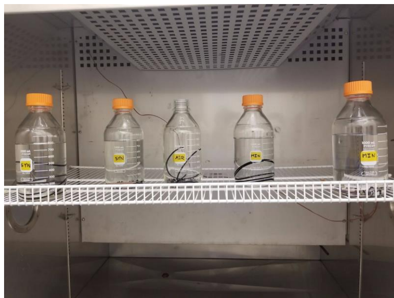
Figure 3.2 Experimental Setup in Environmental Chamber for Thermal Cycle
