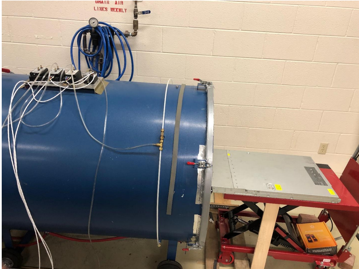
Figure 27 Setup of server for airflow bench testing
