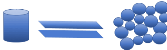
Figure 3-11 Examples of simple pore models (from left to right): cylinders, slits, and voids
