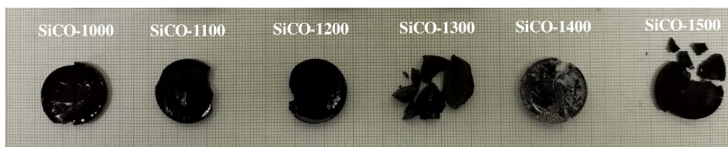
Figure 5-3 Optical images of SiCO ceramics from SiCO-1000 to SiCO-1500
