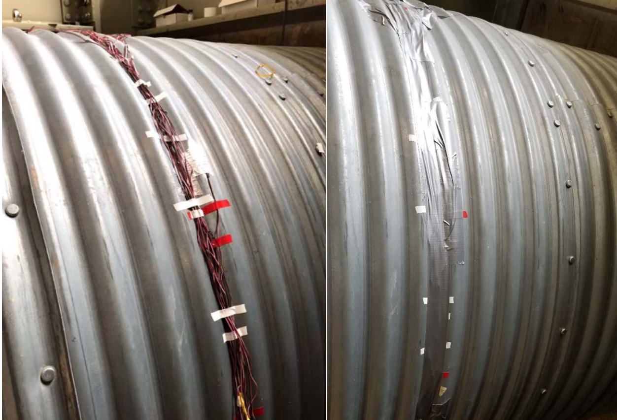
Figure 3-7: Wiring and final duct tape covering over the strain gauges. (source: CUIRE Laboratory)
