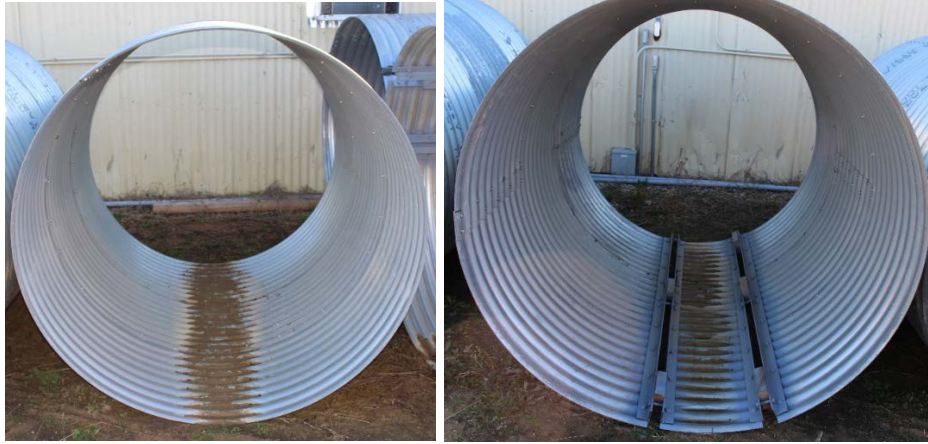
Figure 3-4: Regular CMP (left) and CMP with removable invert (right). (source: CUIRE Laboratory)
