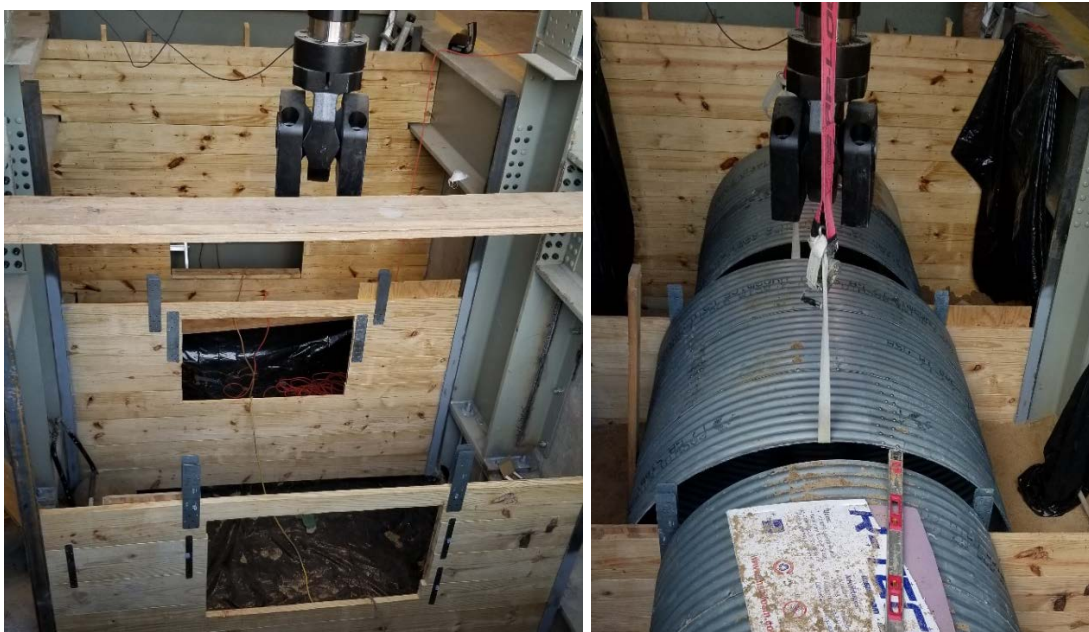
Figure 3-1: Soil box before (left) and after (right) installation of the CMPS (source: CUIRE Laboratory)
