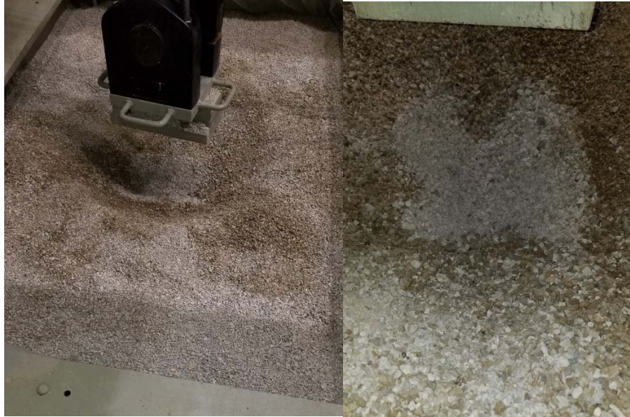
Figure 3-10: Bearing failure of soil below the load pad. (source: CUIRE Laboratory)
