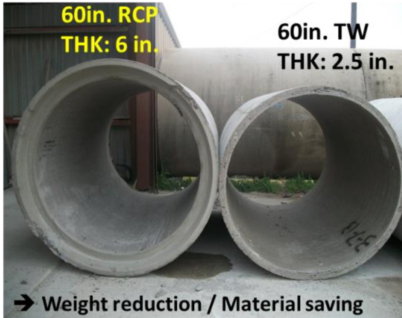
Figure 3.2 Comparison between RCP and TW pipe (ID: 1520mm=60in.)
