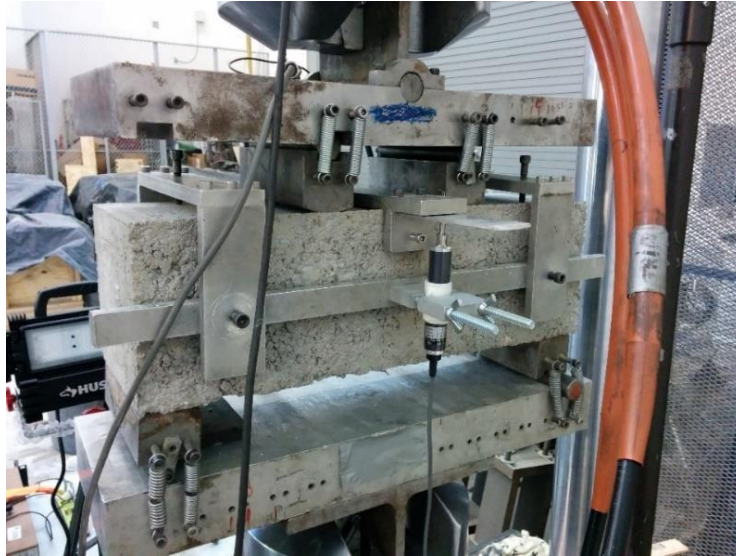
Figure 4.10 LVDT and jig arrangement to measure the mid-span deflection four-point bending test
