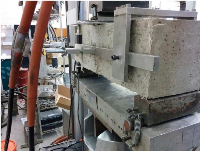
Figure 4.7 the rectangular jig to obtain the net deflection
