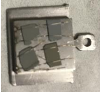
Figure 6-1: Sample set up for HAXPES measurement.
