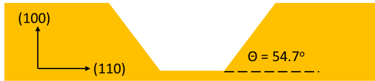
Figure 7-6: Anisotropic Si etch with KOH. The different etching rate in [100] and [110] directions will create a 54.7° slope.
