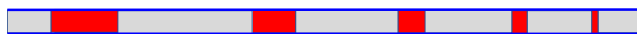
Figure 4- 1 Illustrative multi-segment marker consisting of fluorocarbon segments (gray) and immiscible conductive segments (red) consisting of a salt solution or a liquid metal. Note deliberately differing segment lengths. The terminal FC segments are not used for measurement.
