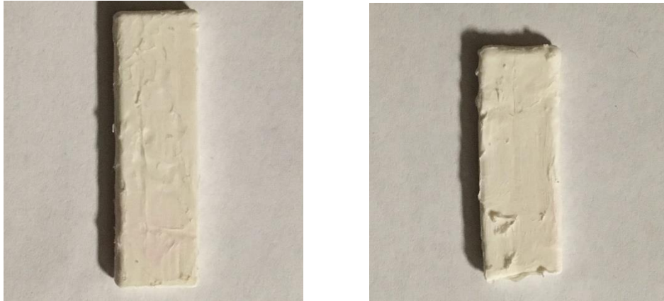
Figure 2.5 Examples of excessive dipping with (left) DCM and (right) chloroform.
