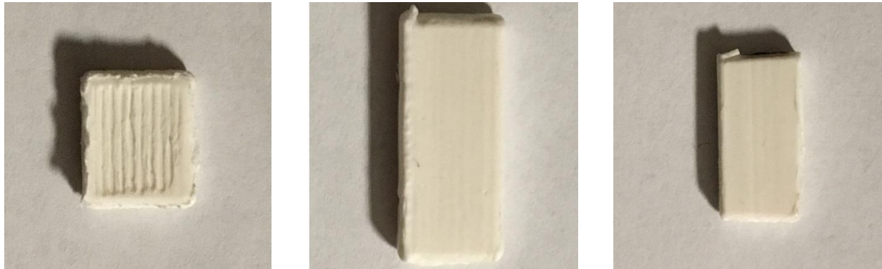
Figure 2.3 PLA samples after vaporization with (left) ethyl acetate, (middle) DCM, and (right) chloroform.
