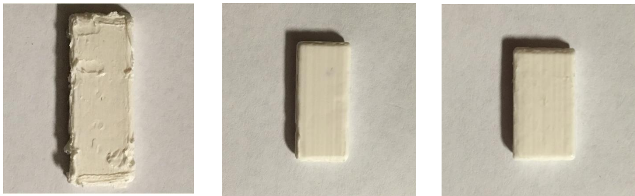
Figure 2.4 PLA samples after dipping with ethyl acetate (left), DCM (middle), and chloroform (right).
