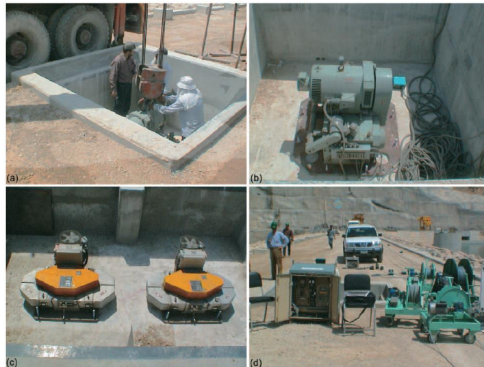
Figure 2-19: Vibration generators used for forced vibration tests on Masjed Soleiman Dam (after Jafari and Davoodi 2006)
