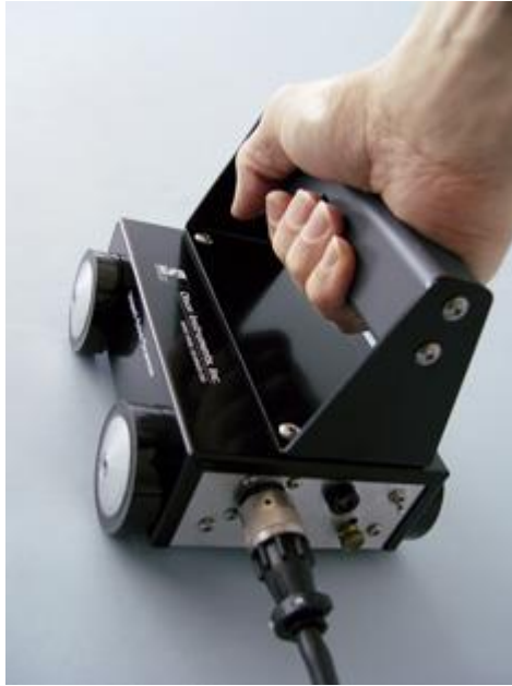
Figure 2.12 Handheld impact-echo non-destructive testing equipment (Hoensheid et al. 2012)
