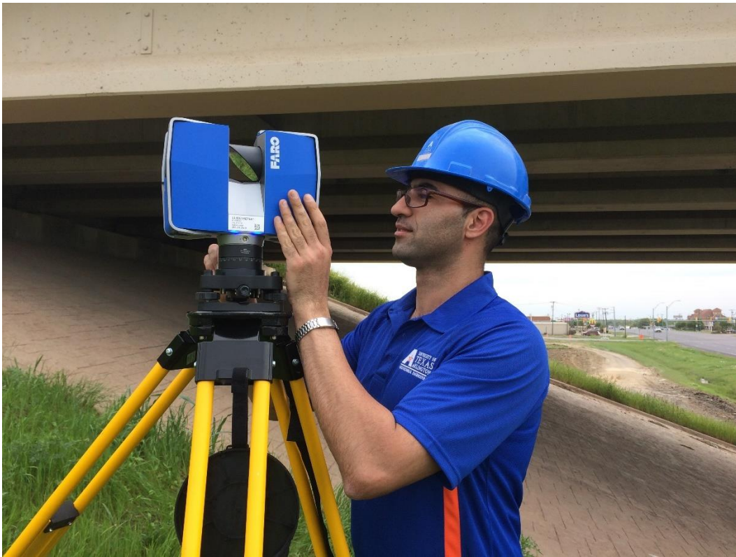
Figure 4.8 Long range 3D TLS LiDAR survey
