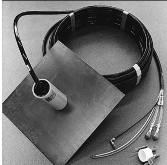
Figure 2.8 A typical type of settlement cell (Indicator 2004)
