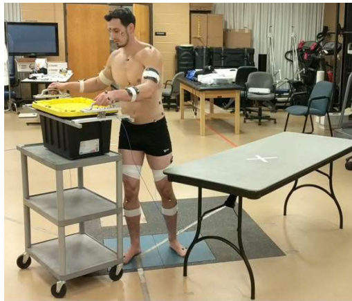
Figure 11 : Asymmetrical Lifting Task picking up from the front along sagittal plane ground level releasing 90-degree angle from pickup
