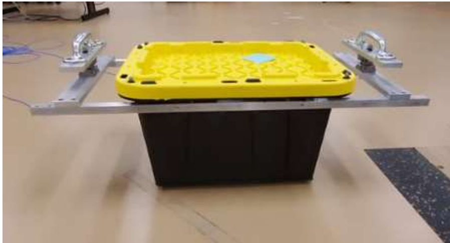
Figure 3: Customized Lifting Bin instrumented with three-dimensional force transducers PCB model 261A01 (PCB Piezotronics, Inc, Depew, NY) which were also sampled at 1000 Hz.
