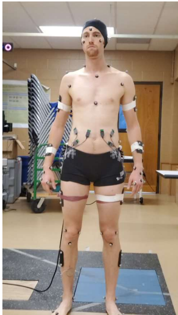
Figure 8: Full Body Front Reflective Markers and EMG Placements On Subjects
