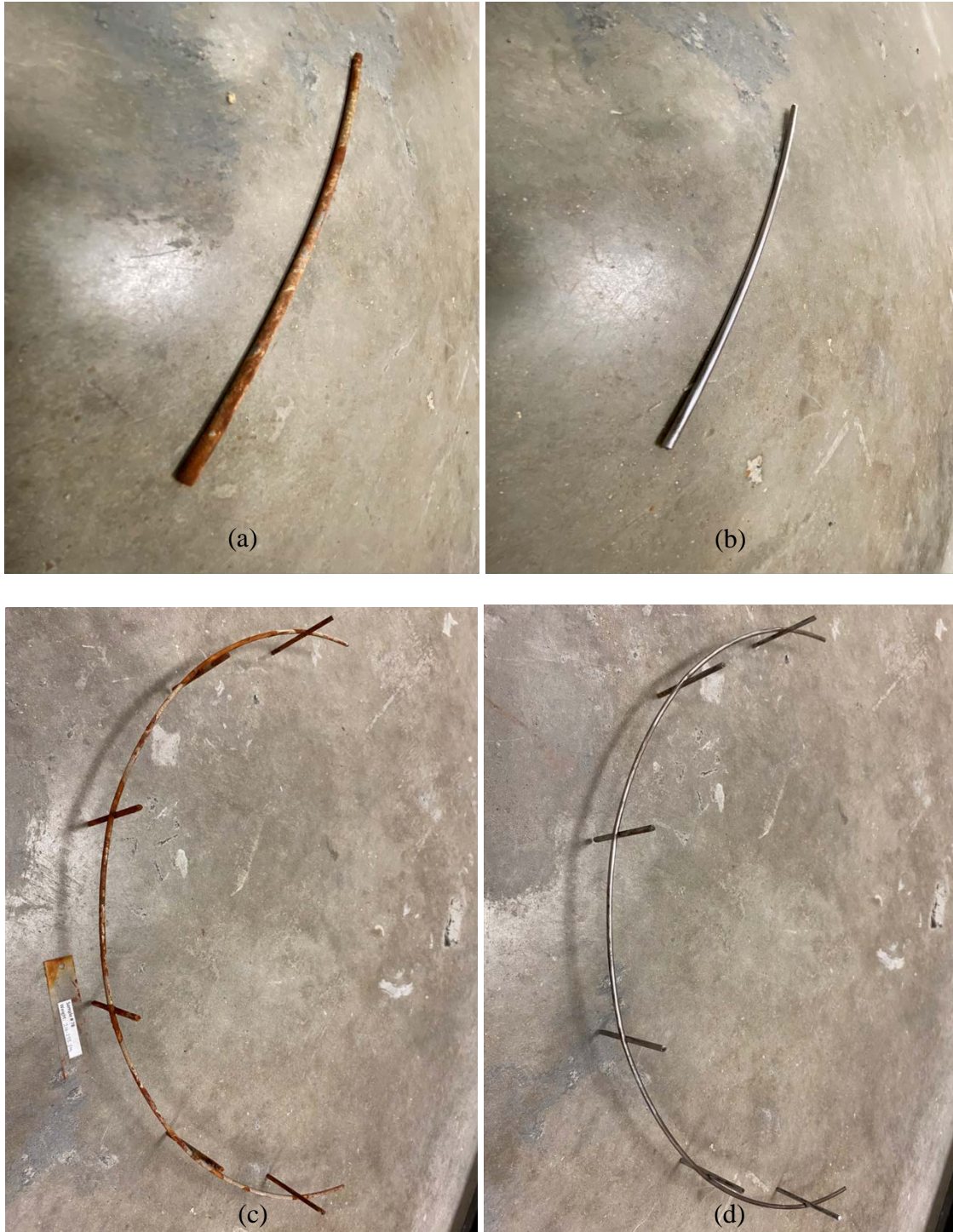
Figure 99: (a) helical bar before cleaning, (b) helical bar after cleaning, (c) half steel cage before cleaning and (d) half steel cage after cleaning.
