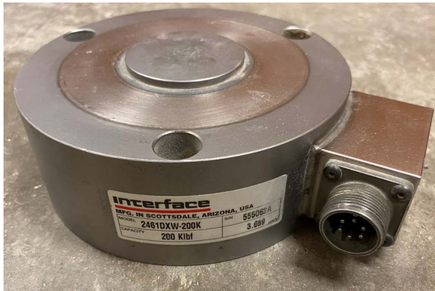
Figure 49: Load cell and the calibration values shown on the sticker.
