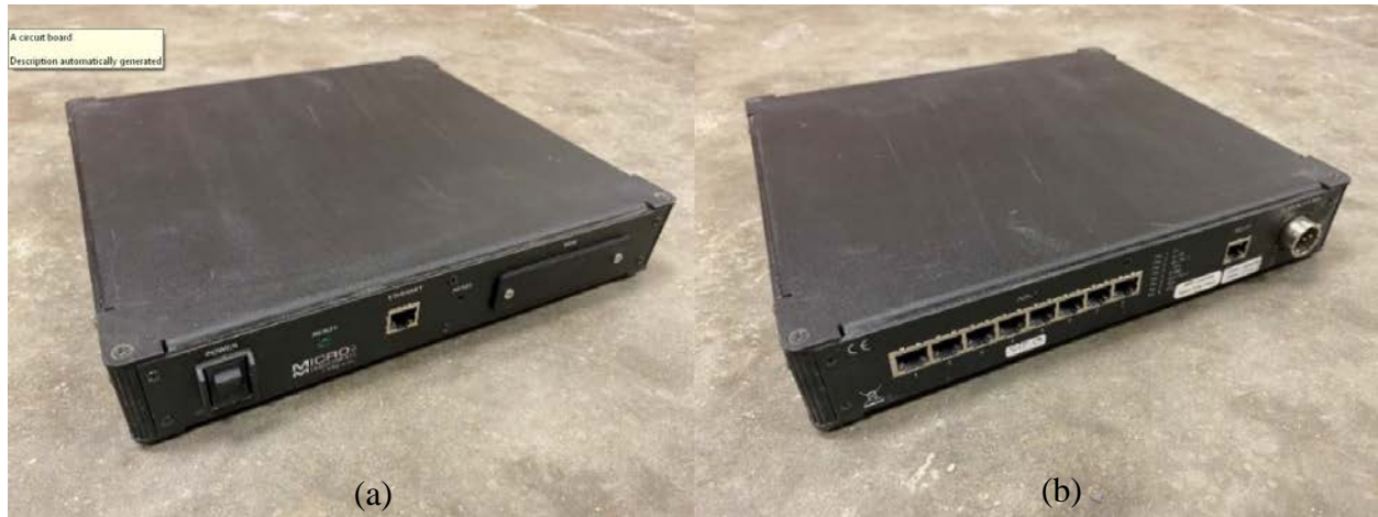
Figure 52: Data Acquisition System, System 8000, (a) front panel and (b) back panel.
