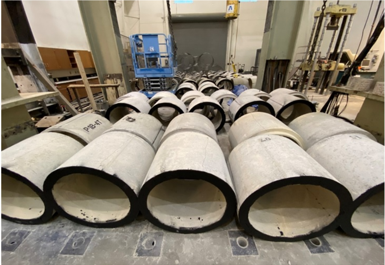
Figure 38: Cut sections of the pipes sealed with rubber sealant.
