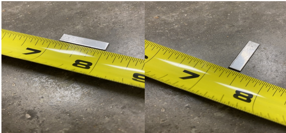
Figure 44: Stainless steel spacer with a thickness of 0.063 inch.
