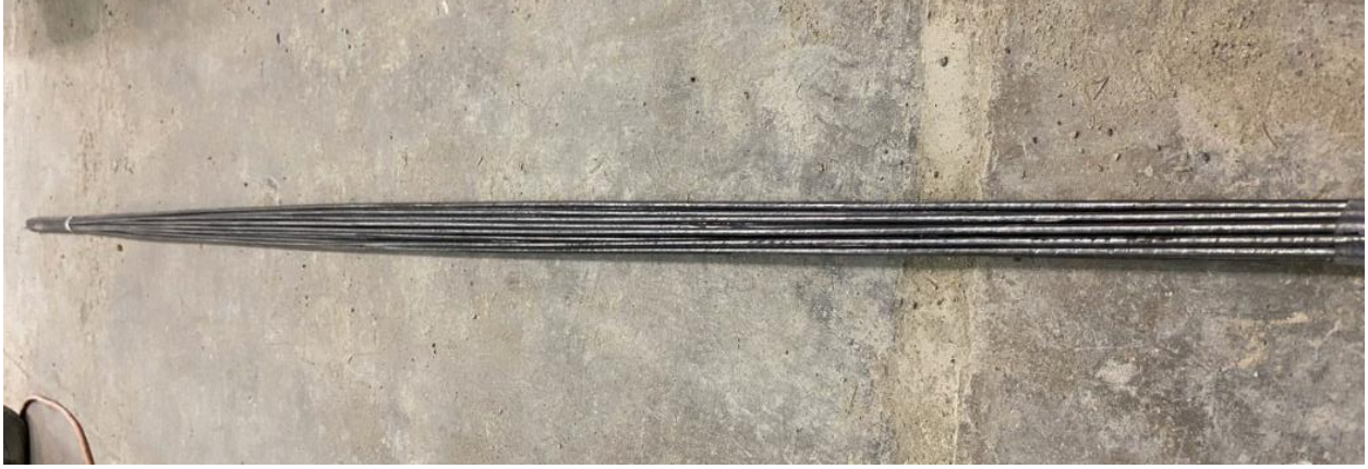
Figure 46: Straightened bars to make tension coupons.
