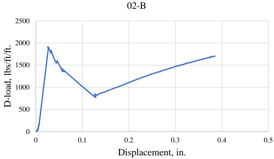
Figure A- 3: Pre-immersion D-load – Displacement Curve for pipe 02-B
