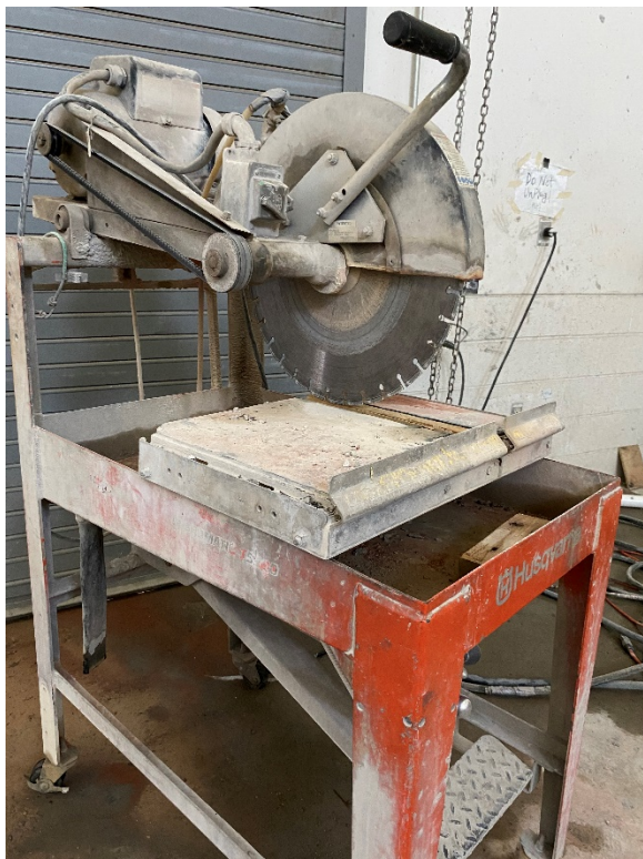
Figure 56: Concrete Saw used to cut SEM/EDX specimens
