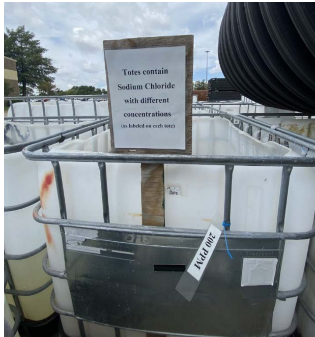
Figure 42: Labels for the contents of the totes and the tags on the totes to indicate the concentration of sodium chloride
