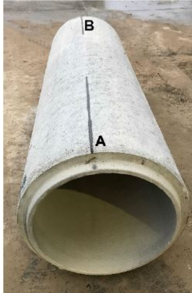
Figure 35: Full length 24 inches reinforced concrete pipe manufactured by Forterra Pipe Plant.
