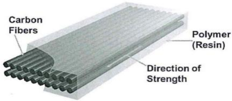
Figure 1-1 Schematic diagram of a CFRP sheet (Yang, 2007)
