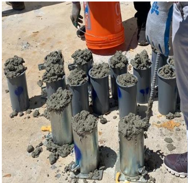
Figure 3-1 Casting of concrete cylinders
