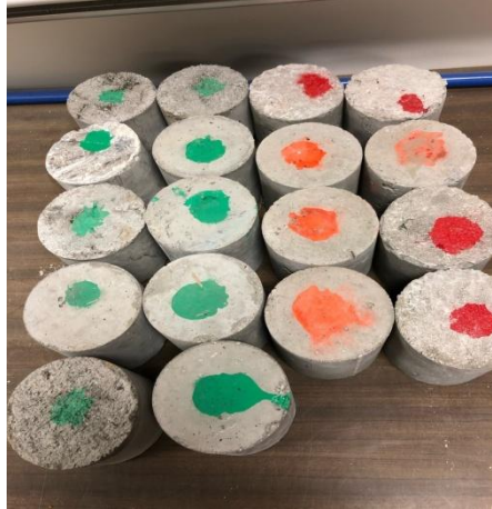
Figure.3-2 Test specimens before CFRP wrapping
