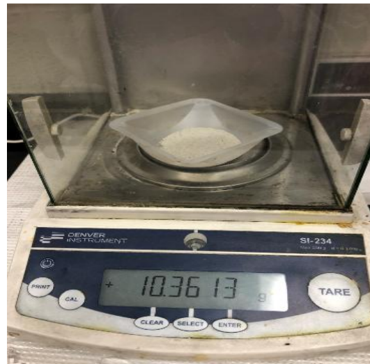
Figure 4-2 Concrete samples drilled using rotary impact drill, collecting approximately 10 g of powdered material.
