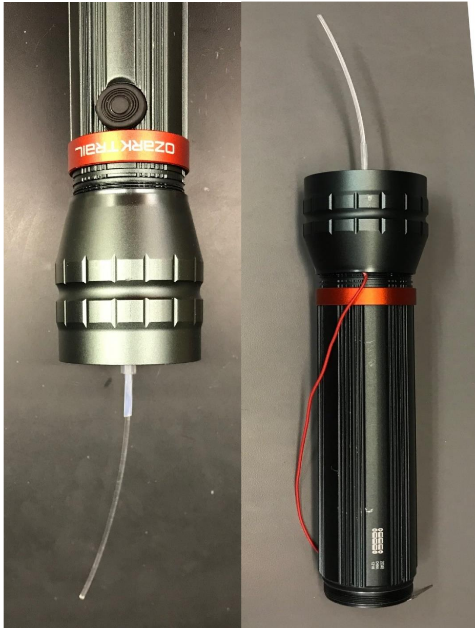
Figure A-S3 The delivery fiber is firmly coupled to the LED chip through a hole in the front plastic face. The LED lead wires are brought out through the sides to connect to a standard power supply.
