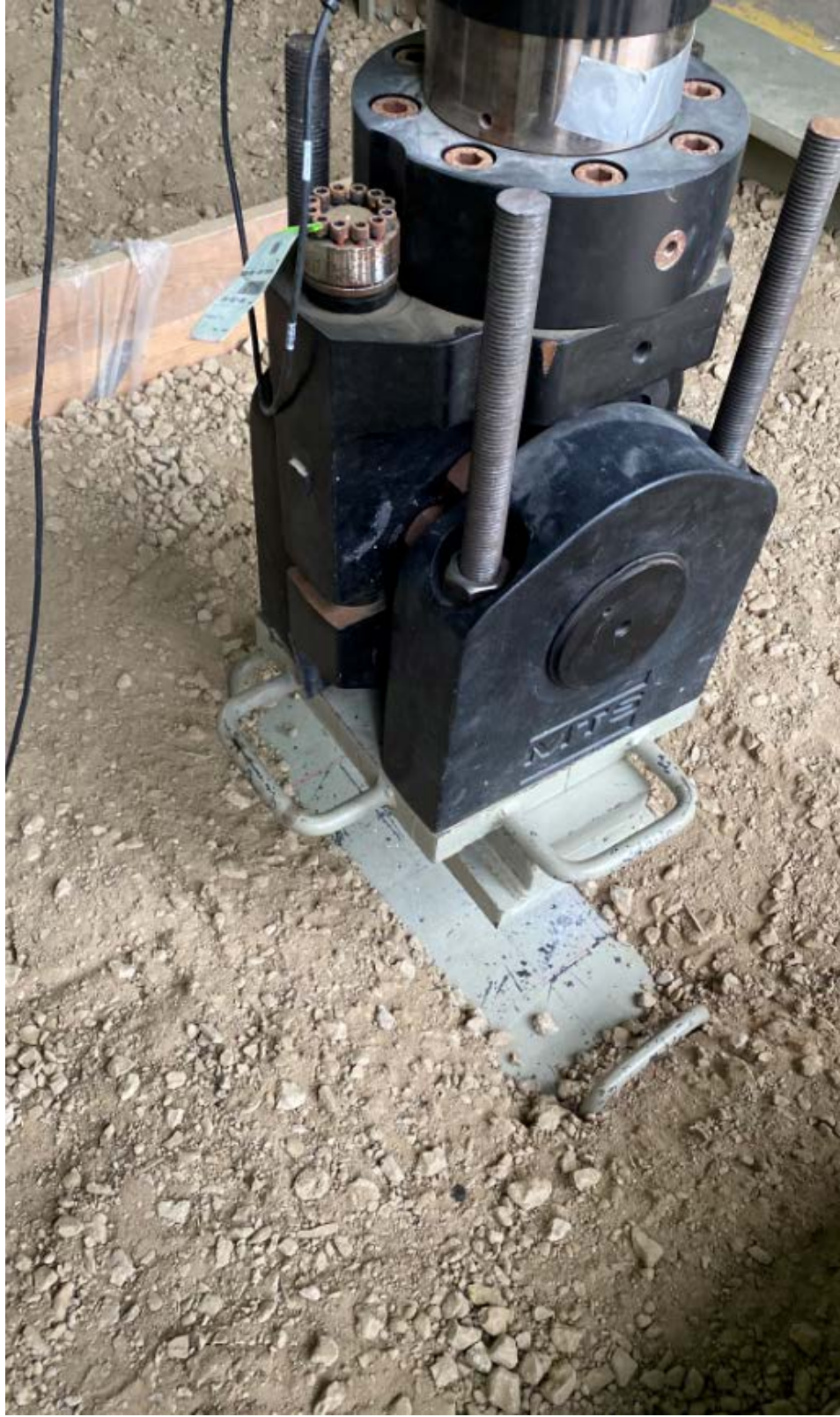
Figure G-27. Load pad penetration in to the soil at the end of test.
