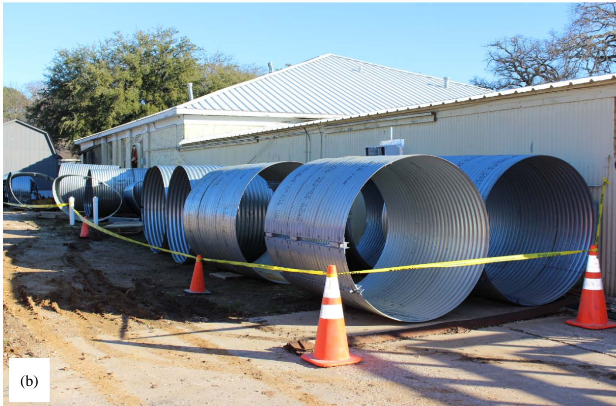
Figure 3-12. Intact and invert-cut CMP samples: (a) transportation to laboratory facility, and (b) storage area.
