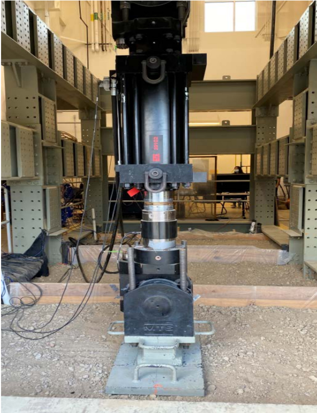
Figure G-26. MTS hydraulic actuator applying a static load over the soil surface.
