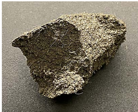
Figure 3-33. GeoCast© mortar with its micro fibers.
