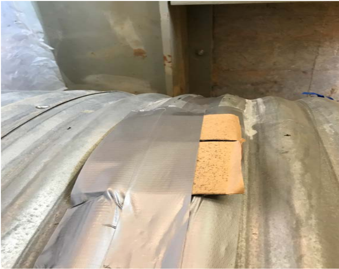
Figure G-13. Strain gauge physical protection.
