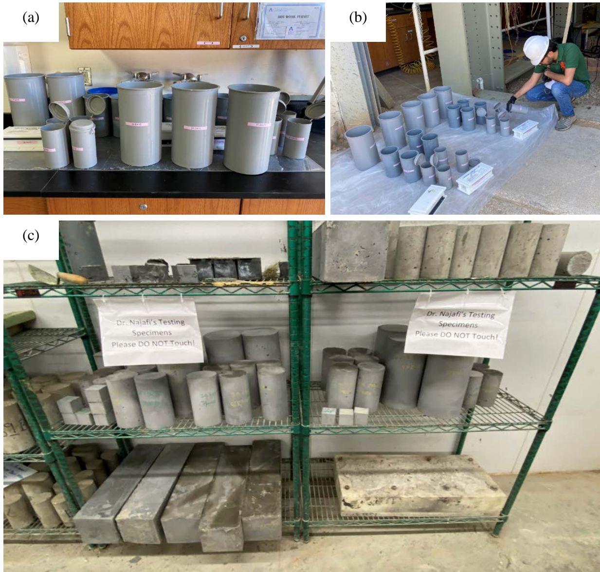
Figure 3-45. Mechanical properties testing samples: (a) compressive testing cylinders molds, (b) mold preparation, and (c) sample storage at a curing room.
