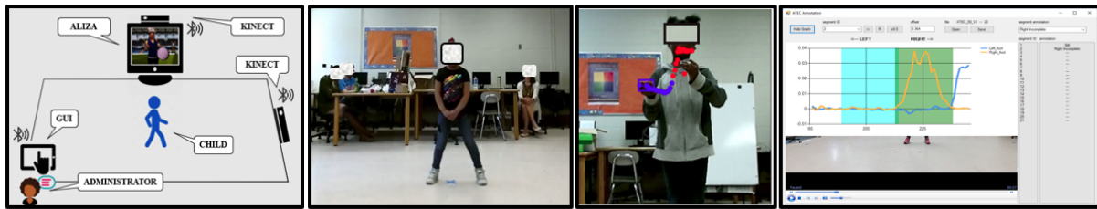
FIGURE 2.2: The ATEC setup includes two Kinect cameras, a large screen and a tablet interface for the administrator. Administration takes place in classroom environments. Annotation software was developed to enhance manual scoring and annotate the collected data, given the task rules and the cognitive measures to be assessed.
