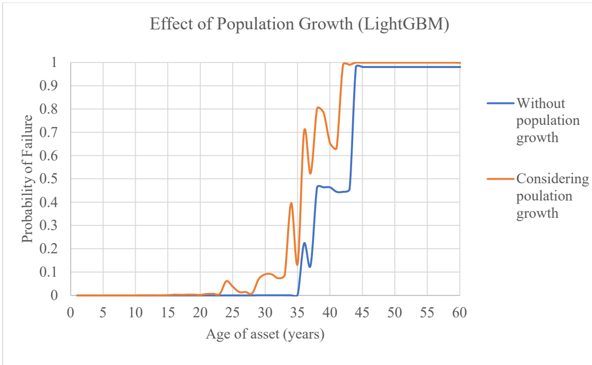
Figure 5.11: Influence of population growth on probability of failure (based on LightGBM model)
