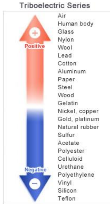
Figure 1.16: Triboelectric series representing the relative electron affinity between materials [98].
