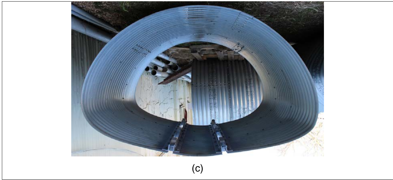
Figure 4-4 Circular CMP samples for control test: (a) intact 60 in. circular CMP, (b) invert-cut 60 in. circular CMP, 47 × 71 in. and (c) invert-cut CMP arch.
