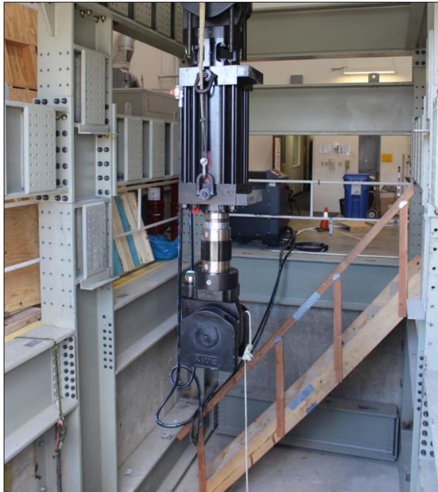
Figure 4-30 The 330-kip MTS actuator hydraulic actuator attached to a reaction steel frame located at the CUIRE Laboratory at the University of Texas at Arlington.
