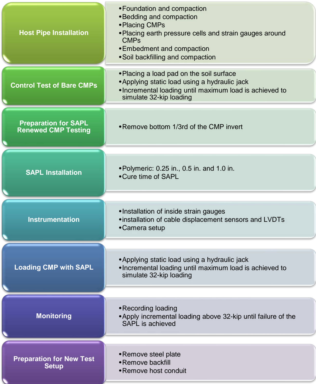
Figure 4-2 Overview of soil box testing steps.
