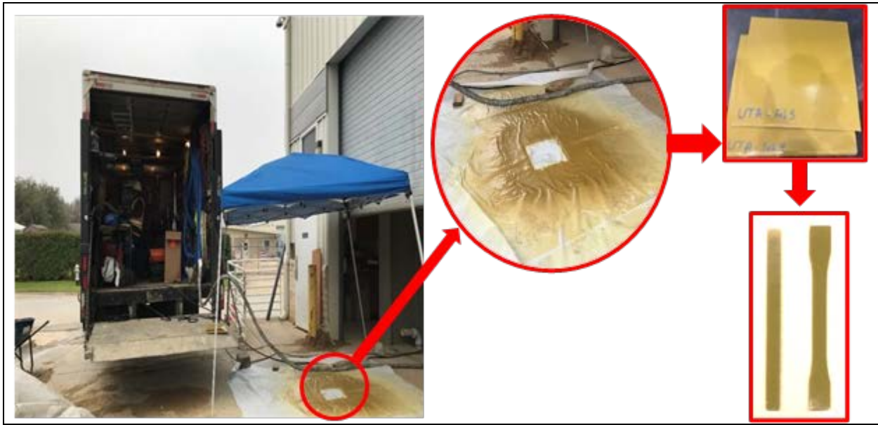
Figure 4-20 Plate sampling from the SAPL batch to provide material test samples for arch CMPs test setup.
