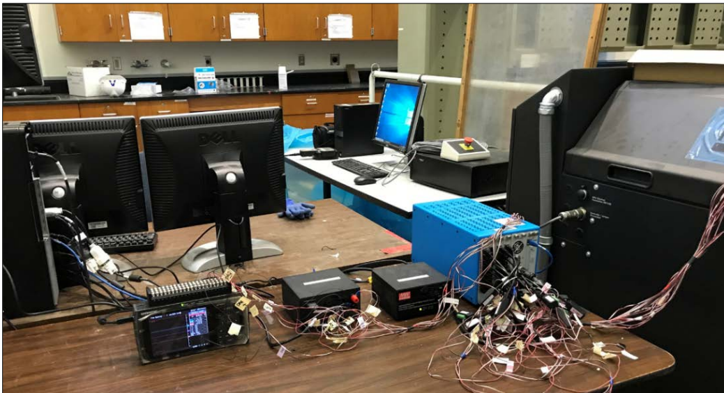
Figure 4-22 Strain gauges connected to a data acquisition system (DAQ).
