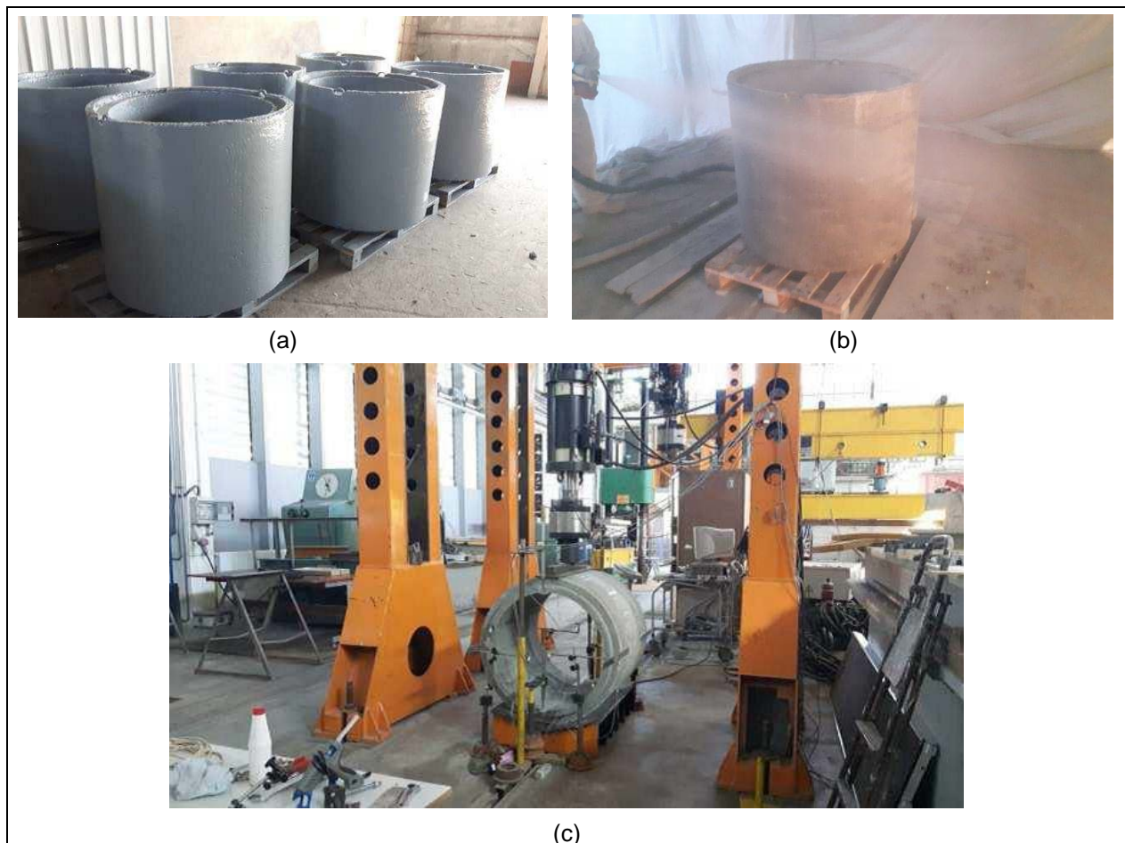
Figure 2-4 Dead-load testing of reinforced concrete pipes (RCPs) renewed with polymeric SAPLs: (a) tested concrete rings covered by polyurea coating, (b) spraying polyurea coating system on concrete ring, and (c) D-load testing frame (Szafran and Matusiak 2017).
