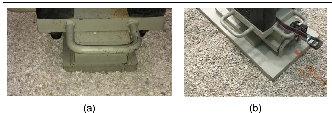
Figure 4-31 Steel load pad: (a) 10 × 20 in., and (b) 20 × 40 in. pad size.
