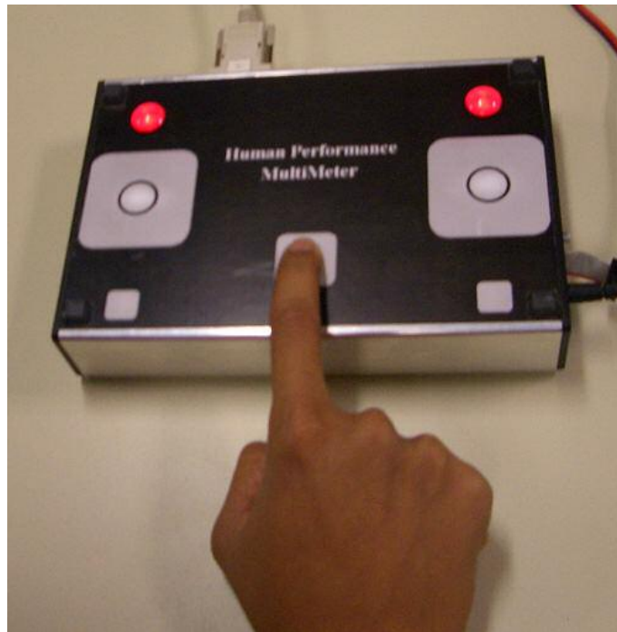
Figure 4.2 Picture of the subject executing the Visual Auditory Information Processing Dexterity Test (GTA 11). Subject has finger on HOME sensor. Both LEDs are lighted (Situation 4)
