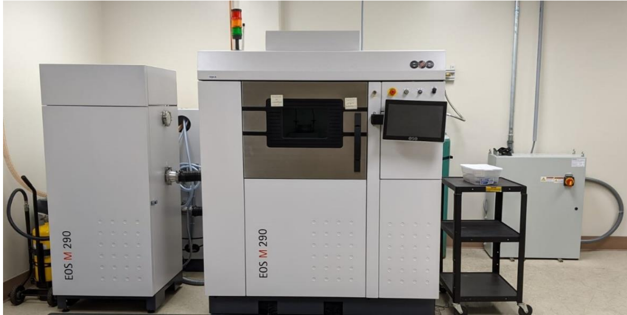
Figure 5: EOS M290 machine with a 400 W fiber laser.
