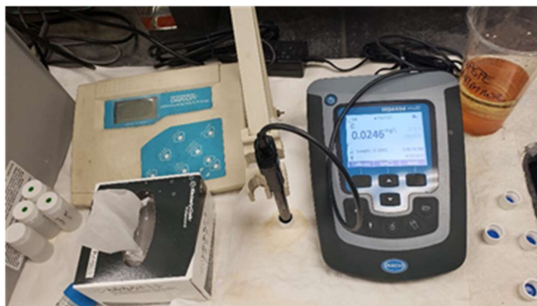
Figure 2-1: Fluoride Intellical F121 electrode probe coupled to a Hach HQ 440D base.
