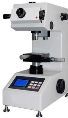
*Figure 26. LECO LM 300 AT Micro Hardness Tester*
