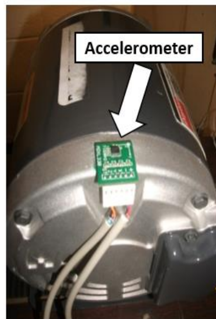
Fig. 4. 8 Tri-axial Accelerometer Measurement on the Motor Housing
