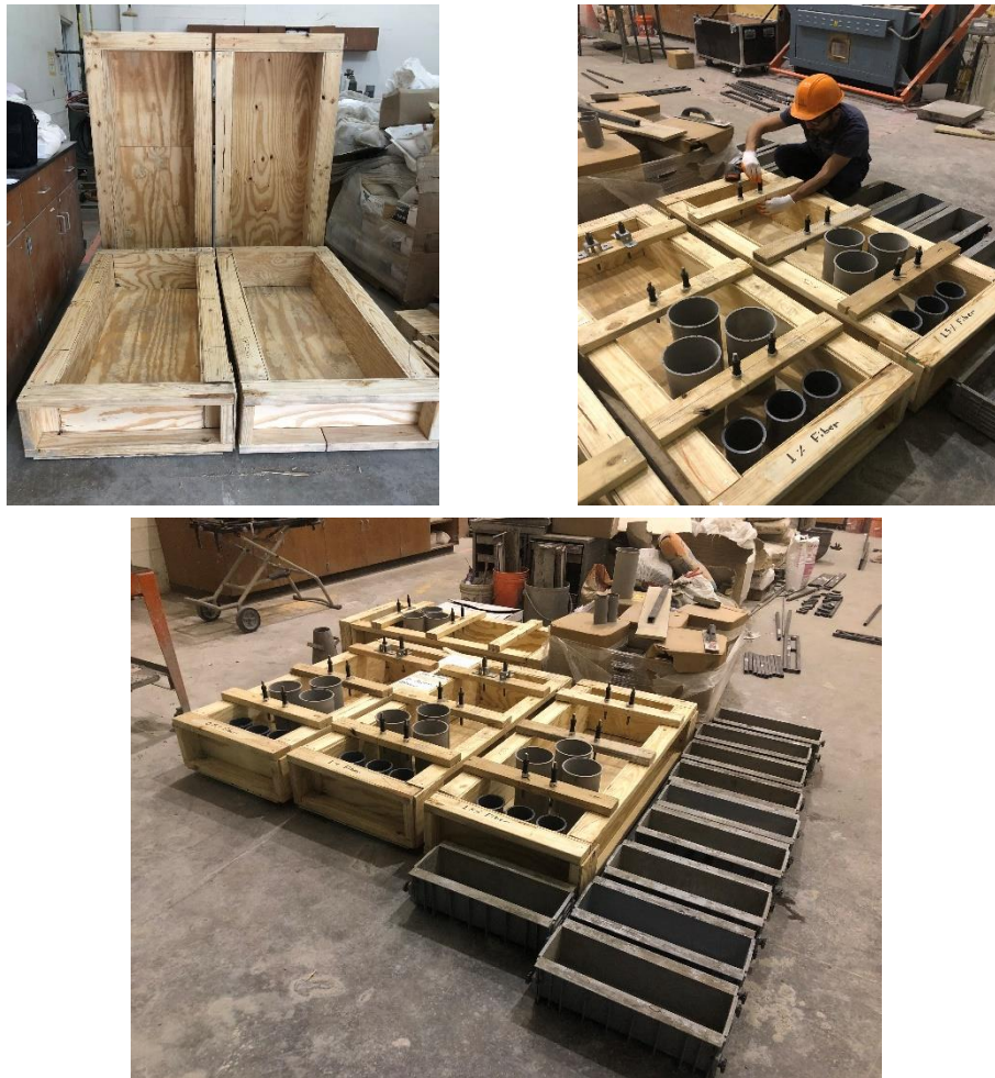
Figure 3.4 Stages of Timber Formwork Specimens
