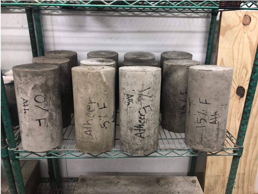
Figure 3.11 Concrete Specimens in the Curing Room
