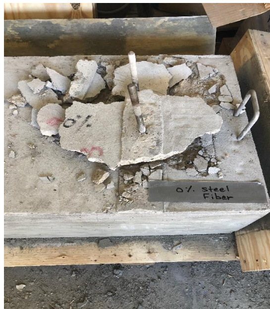
Figure 3.24 Concrete Breakout Failure (0.0% SFRC)
