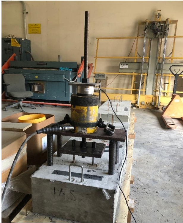
Figure 3.21 Pull-Out Test Set-Up (On-Site)
