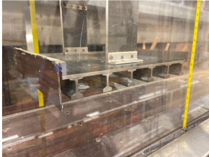
Figure 20- Flat plat debris test arrangement
