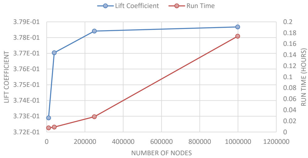
Figure 4: NACA 65-210 Grid Independence – Lift Coefficient
