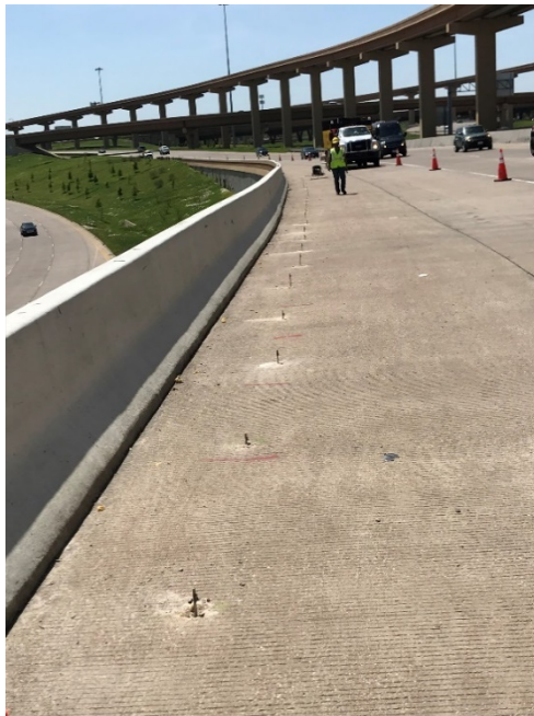
(b) Inserting and hammering the electrodes
