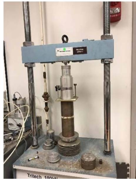
(b) Compacting soil sample
