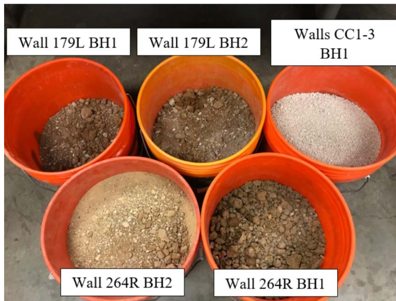
Figure 4-42 Backfill soils obtained from different boreholes
