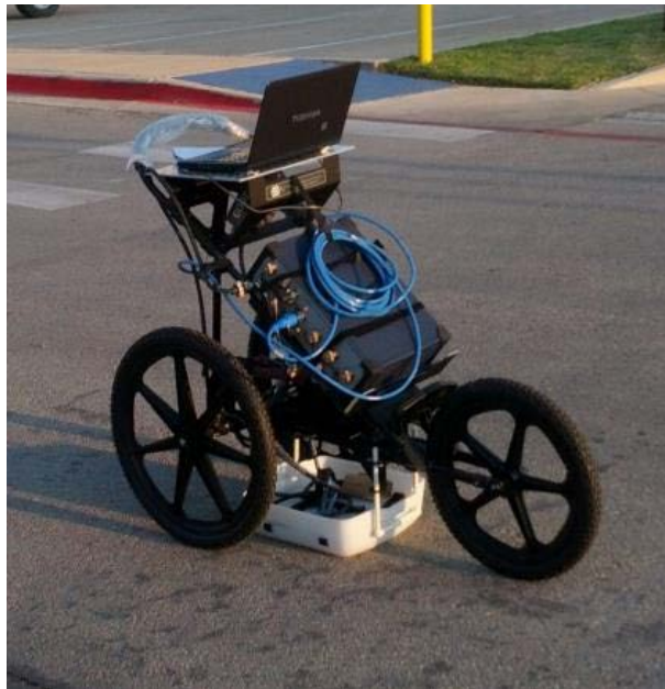
Figure 4-14 GPR machine (Riad 2017)
