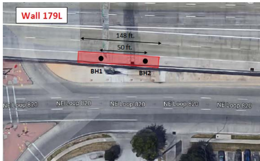
(b) Borehole locations at Wall 179L
