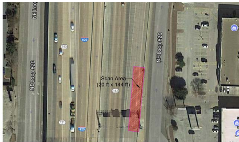
Figure 4-15 Scan area using GPR at Wall 179L
