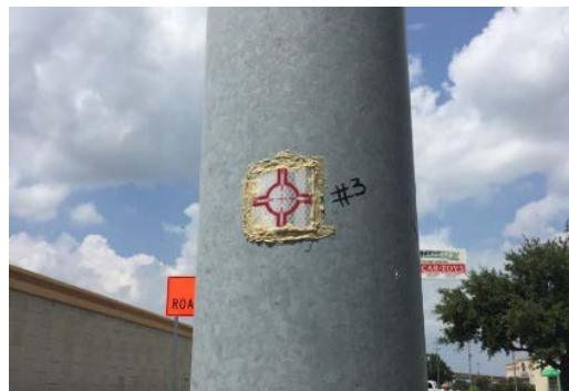
Figure 4-3 Target used as a back sight placed on a light pole
