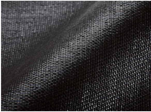
(c) Geosynthetic sheet
