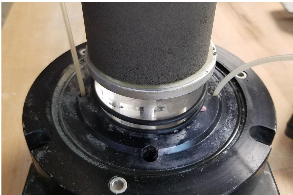
Figure 3-8 Specimen on top of the modified platen
