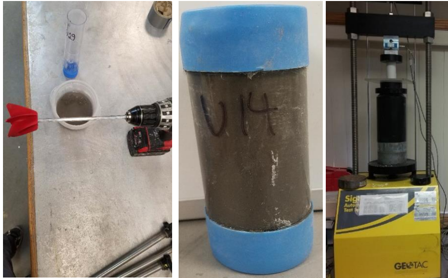
Figure 3-5 a) Rubber blade attached to an electric drill, b) poured materials in mold, and c) tailings specimen in the UCS test setup
