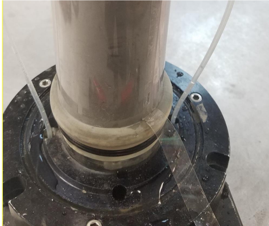
Figure 3-10. Temporary mold made using a PVC binder cover
