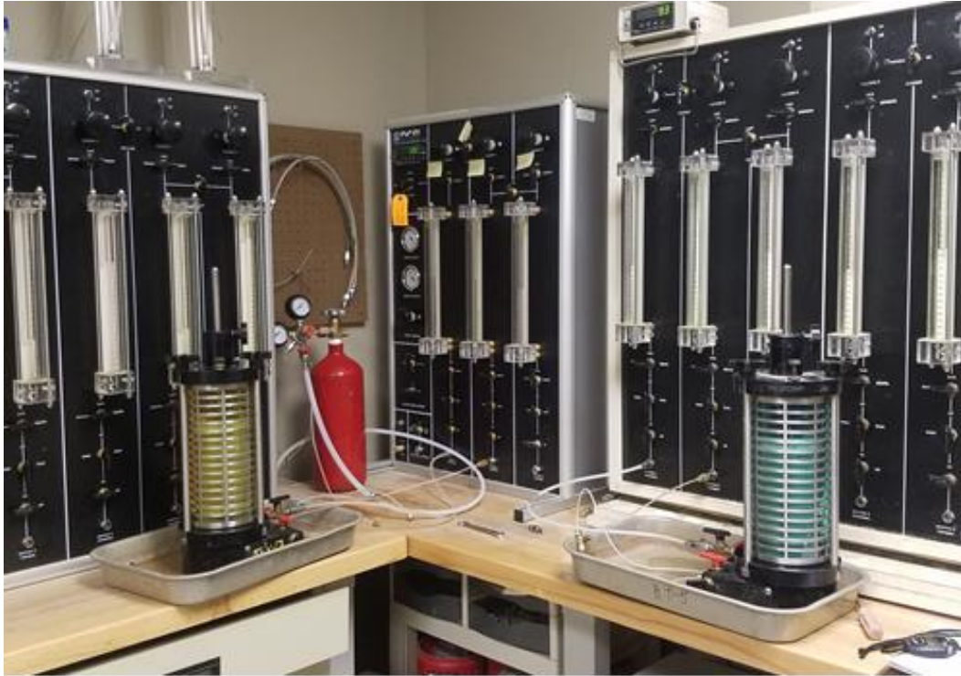
Figure 3-9 Back-saturation and consolidation stations with the CO 2 cylinder
