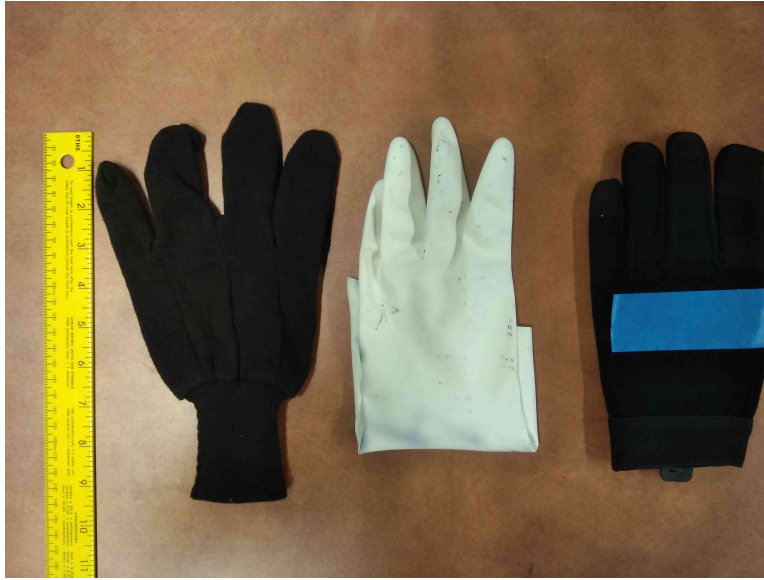
Figure 3.3. Types of gloves: cotton (left), dishwashing rubber (middle) and mechanics (right).
