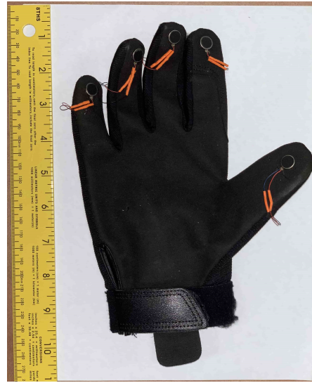
Figure 3.10. Wearable glove Ventral side.
