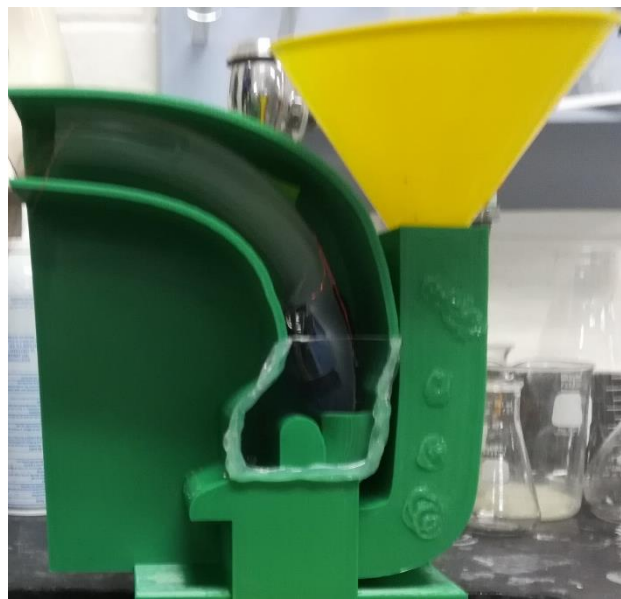
Figure 72: Back profile of LMA with sensors embedded
