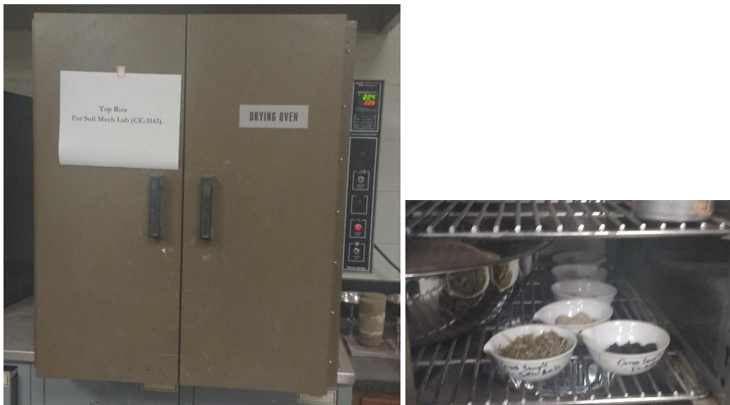
Figure 3.33: Moisture content test of materials in column reactors
