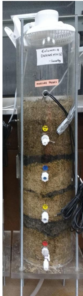
Figure 3.26: Column reactor 4 with grass, biosolids and fly ash
