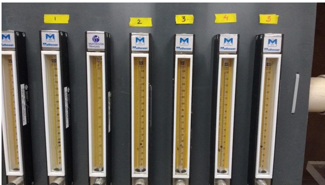
Figure 3.29: Flow meters for controlling flow of inlet gas to the column reactors
