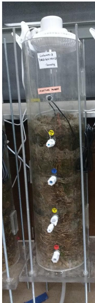
Figure 3.25: Column reactor 3 with grass, biosolids and fly ash
