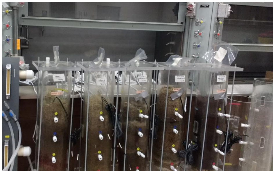
Figure 3.32: Tedlar bag installed on column reactors
