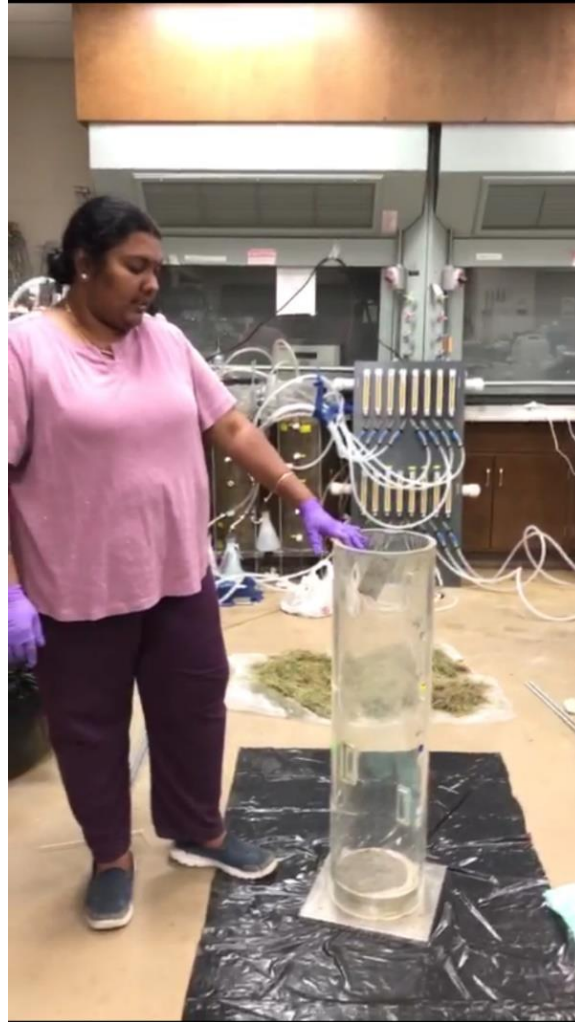
Figure 3.20: setting up reactor to fill biocover material
