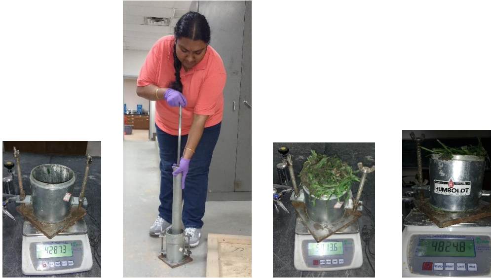
Figure 3.13: Compaction test on the biocover materials
