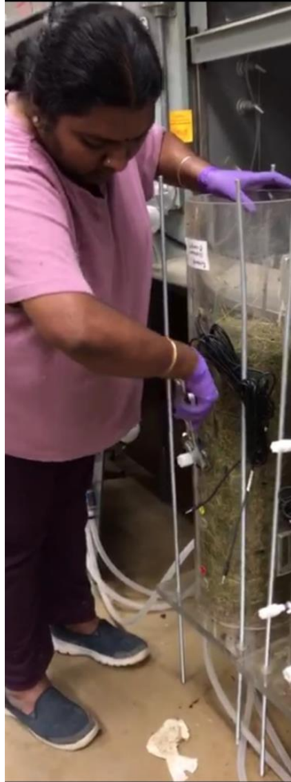
Figure 3.22: Column reactor 1 after setting up
