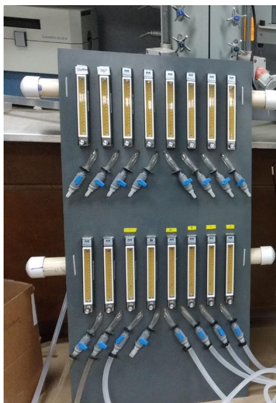
Figure 3.16: Manifold for distributing inlet gas
