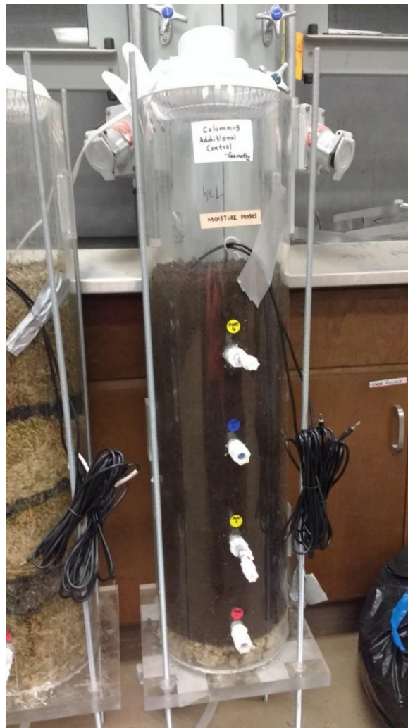
Figure 3.27: Column reactor 5 with compost
