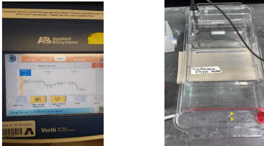
Figure 3.35: Thermal cycling in PCR and gel after adding sample and dye
