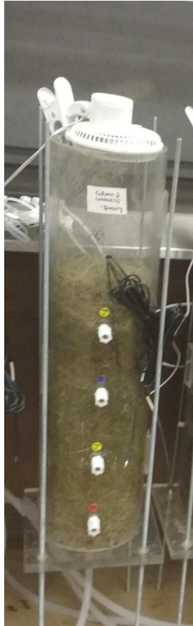
Figure 3.24: Column reactor 2 with grass clipping as biocover material
