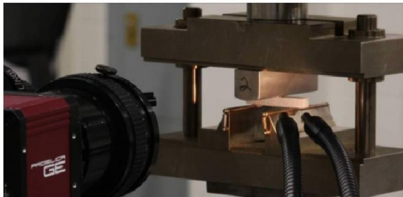
Figure 4. Short Beam Shear Test Setup, showing the fixture, a coupon being tested, and the optical system.
