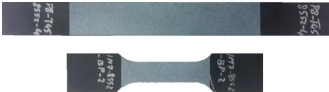
Figure 38. ASTM D3518 Specimens made of IM7/8552: 8-ply straight [\pm 45]_2 s (top) and Dog-Bone [+45_2 / -45_2]_s (bottom) Specimens
