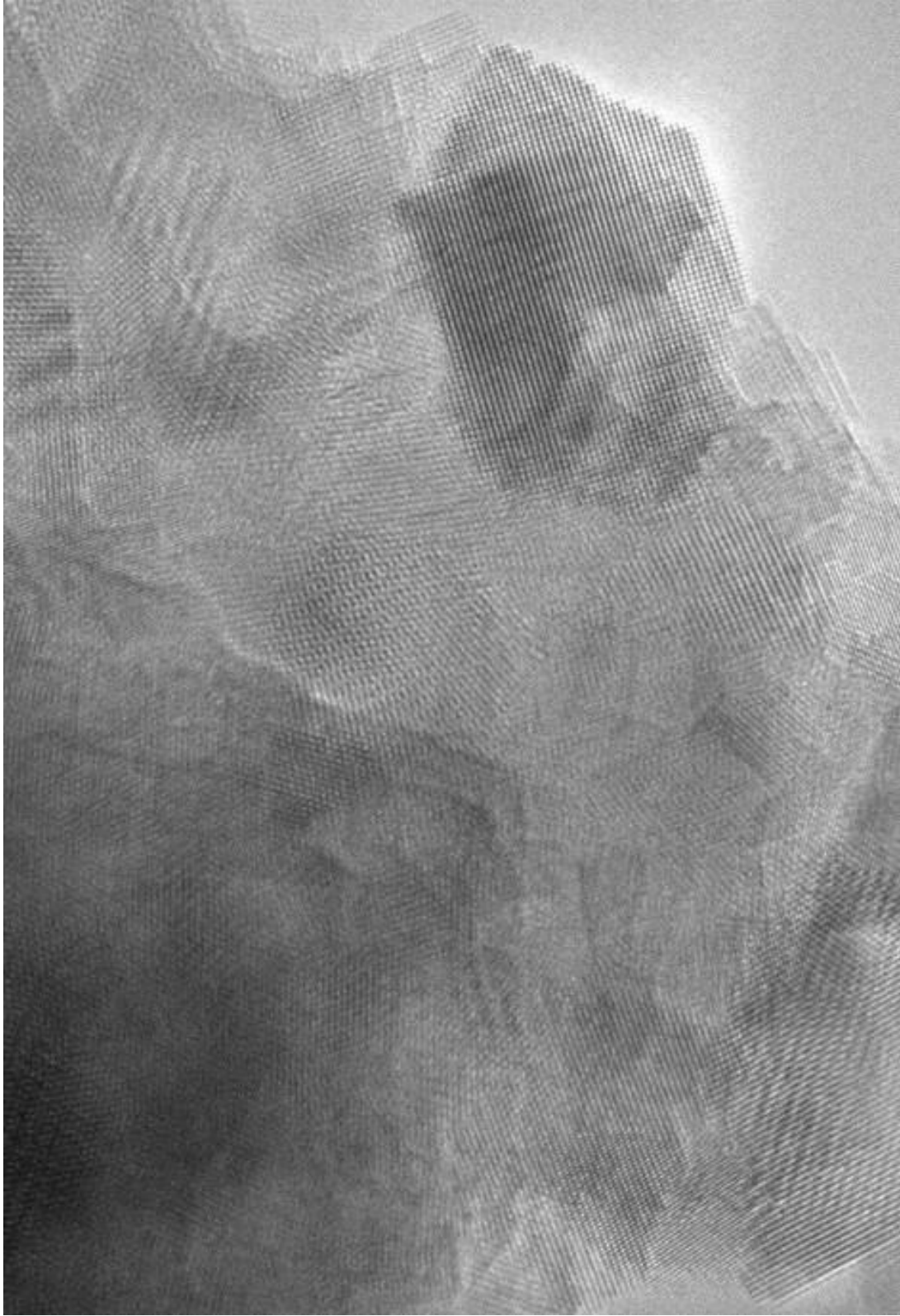
Figure 3.5.9 "Image Number 26" Hitachi H-9500 HRTEM Image of Clinoptilolite over Copper/Lacy Carbon TEM Grid at x750k Magnification
