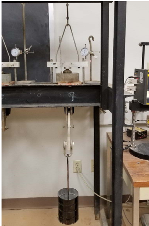
Figure 3.6 1D swell strain test setup
